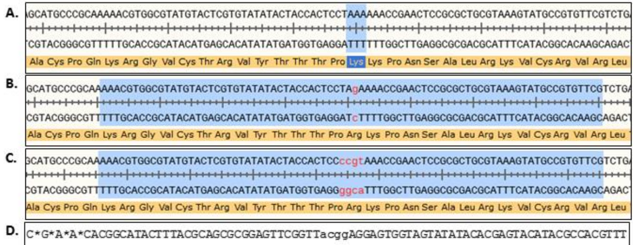
Figure 3. Oligo design for recombineering of the rpsL gene in E. coli . A) The up- and downstream nucleotide sequence of rpsL with the site of mutation highlighted in blue. B) A single bp mutation shown in red causes the substitution K43R. The 80 bp of DNA sequence corresponding to the mutation oligo is highlighted. C) Three silent mutations are shown in red to evade the mismatch repair system. D) Final oligonucleotide design that includes 4 bp mismatches shown in lowercase, 4 phosphorothioate bonds at the 5' end, and targets the lagging strand.
