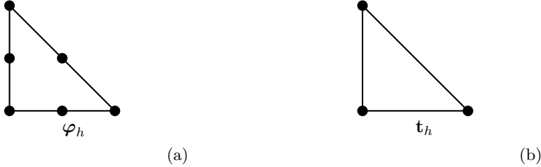
Figure 5: Node locations for k = 2 element for (a) the displacement interpolation and (b) the director interpolation
