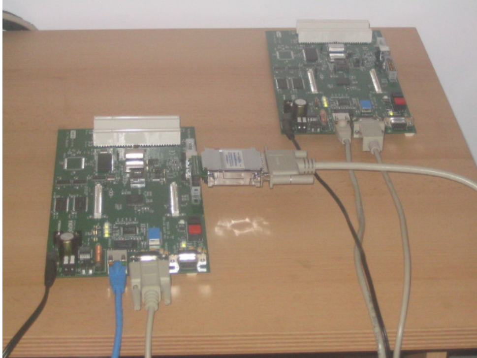
Figure 4 - M5272C3 boards used in the tests.
