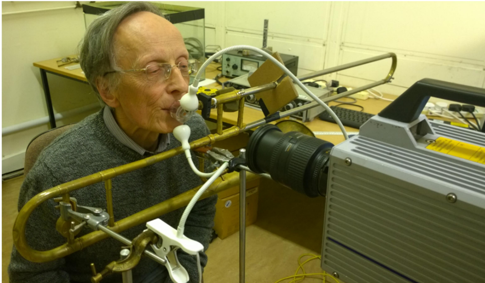
Fig 1. Photographing trombone player's lips showing the high speed camera, the transparent mouthpiece with the trombone body attached to the right side and LED lights.
