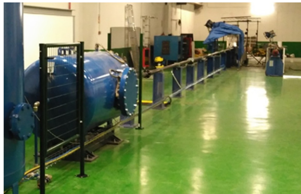
Fig. 5 Gas gun general view at University Carlos III of Madrid facilities.
