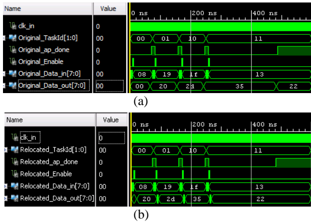
Fig. 7. Output waveforms of Original and Functionality-based relocated circuits. a) Original CORDIC circuit b) Relocated Equivalent
