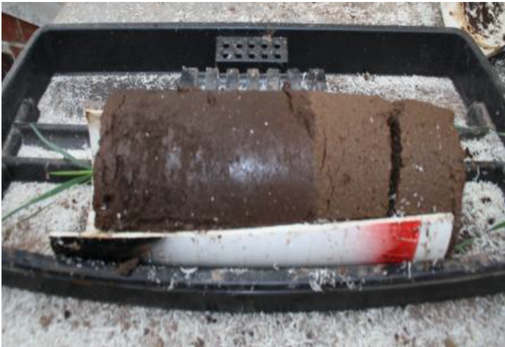
Figure 4: Extracted mixed Soil B3 column; soil layers are distinctly visible (3 Soil B3 layers (darker) overlying 2 Soil A3 layers (lighter)).
