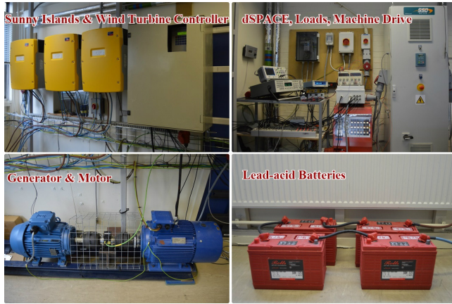
Fig. 6. Hybrid system lab setup equipment
