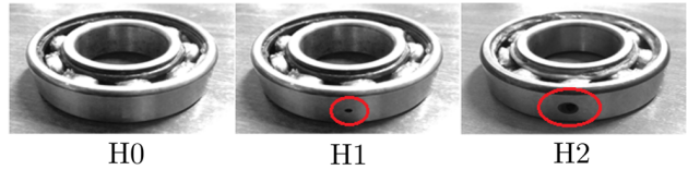
Fig. 4: Bearings Condition: New (H0), 1.6 mm hole (H1) and 5 mm hole (H2).
