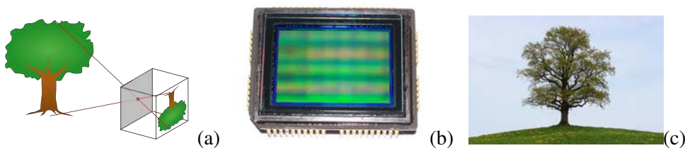
Figure 1.3: Projection camera model: (a) Pinhole model, (b) CCD sensor, (c) Digital image
