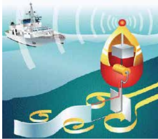
Fig. 1.7. Energy harvesting “eel” concept. (Source: Ocean Power Technologies, Inc.)
