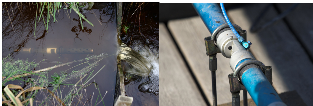
Figure 6. Photograph of the sensors used in the study. Sensors based on ultraviolet-visible (UV-VIS) spectroscopy (left) used to measure turbidity, nitrate-nitrogen ( \text{NO}_3\text{-N} ) and dissolved organic carbon (DOC) in the Lepsämäenjoki River and the wetland studies. A YSI sensor (right) monitoring turbidity, conductivity and temperature in front of a V-notch weir in a small field ditch at the gypsum application study site (left: Lepsämäenjoki River monitoring site, Nurmijärvi 21.3.2007, right: Nummenpää ditch, Nurmijärvi 14.11.2011)
