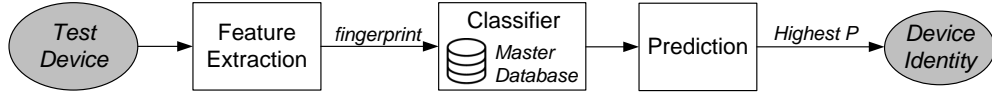
Figure 6: Prediction phase - Device identification. Feature extraction generates a fingerprint with the packet sequence of the test device. Then it is subjected to the classifier which use a master database to provide a list of predictions. The device-type related to the highest probability ( P ) is predicted as the type of the test device.
