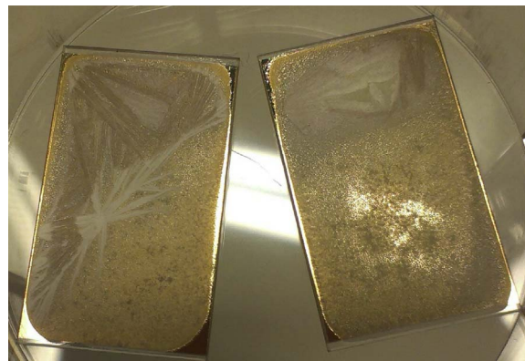
Fig. 2. Au leaching of SPR chips due to LiCl in the 0.1% chitin DMA/5% LiCl solution. White areas are void of gold.
