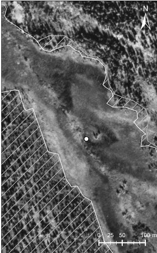
Fig. 1. Aerial photograph of the measurement site. The measurement mast is indicated by a white dot. The white lines show the limit between the open fen and forest areas (hatching = peatland; no hatching = mineral soil).
