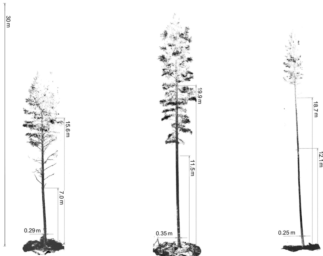
Figure 2. Examples of TLS point clouds of sample trees in this data set. The diameter at breast height (DBH) is indicated horizontally at breast height level (1.3 m from the ground). Height of the lowest dead branch ( H_{db} ) is indicated vertically with the inner right-hand-side number. Length of the saw log section ( L_{log} ) is indicated vertically with the outer right-hand-side number. (Left) A sample tree on plot 3, DBH 0.29 m, H_{db} 7.0 m, L_{log} 15.6 m. (Middle) A sample tree on plot 2, DBH 0.35 m, H_{db} 11.5 m, L_{log} 19.9 m. (Right) A sample tree on plot 4, DBH 0.25 m, H_{db} 18.7 m, L_{log} 12.1 m.
