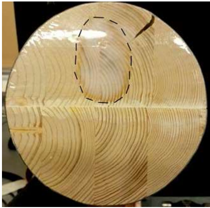
Figure 9: Photograph of the specimen after the experiment, bottom view. The border of the visually observed wetted area in the bottom surface is marked with a dashed line.
