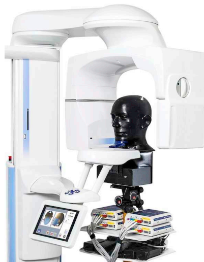
FIG. 2. The MOSFET measurement system with four TN-RD-16 reader modules, RANDO phantom, and ProMax 3D MID CBCT device.
