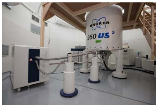
Figure 2: 950 MHz NMR spectrometer Bruker Avance III HD for high resolution spectroscopy in liquids
