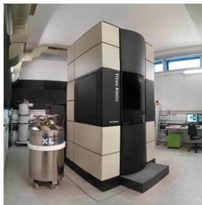
Figure 1: TEM microscope FEI Titan Krios equipped with a direct detector and an energy filter with a 4k CCD camera
