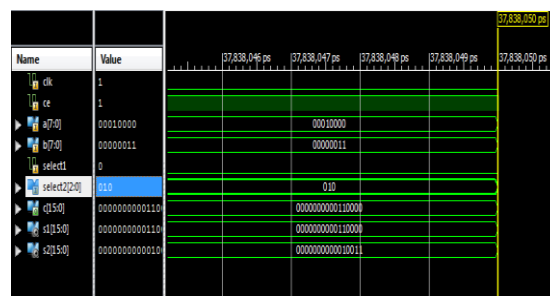
Fig.13. Simulation Result of 8x8 Vedic Multiplier
