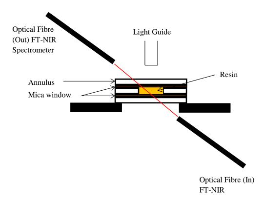
**Figure 2.7.** Experimental setup for laboratory based real time FT-NIR measurements. The resin samples were cured for more than 300 s at varying light intensities whilst undertaking FT-NIRS to quantify the degree of conversion.
