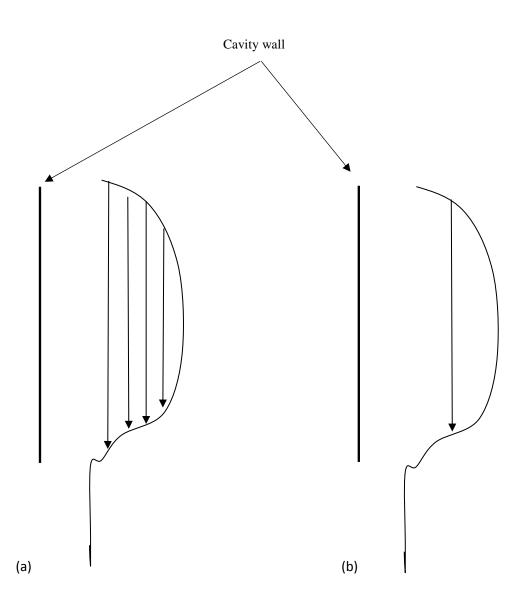
**Figure 7.1.** (a) Schematic of a tooth fin section showing the regions mapped by successive SXRD line scan measurements. (b) A single line scan measurement used to acquire sufficient statistics for each polymerisation regime. The solid black line represents the boundary of the cavity wall.
