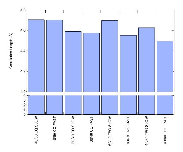
**Figure 4.9.** Final correlation lengths (peak (d),  $q \sim 1.4 \text{ Å}^{-1}$ ) for the each resin specimen post-polymerisation
