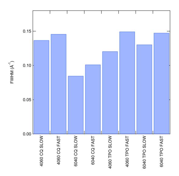
**Figure 4.7.** Full width at half maximum (FWHM) for the scattering peak located at  $q \sim 0.6 \text{ Å}^{-1}$ , post photo-polymerisation for the respective resin blend specimens.
