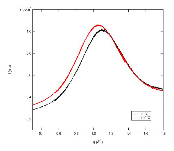
**Figure 5.2.** X-ray scattering of a 40/60 wt % (Bis-GMA/TEGDMA) resin disc sample initiated with TPO. At 20 °C the scattering peak (black line) is located at approximately 1.14 Å<sup>-1</sup>, but moves to lower q (red line), indicative of an increase in the correlation length.
