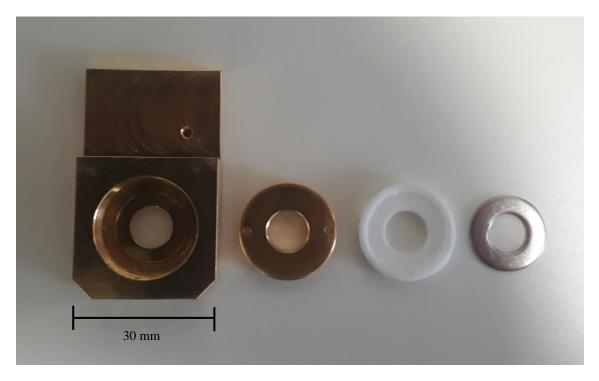
**Figure 2.5.** Liquid containment cells used for *in-situ* polymerisation simultaneous to X-ray scattering measurements. Liquid resin is stored inside a metal washer with mica windows, which is fixed into a PTFE washer that is housed within a brass annulus.
