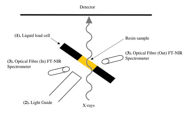
**Figure 3.1.** Real time SAXS measurements of dental resin composites polymerised in-situ on the I22 beam-line (1) liquid resins loaded in to a sample rack in the path of impinging X-rays, (2) A liquid light guide instigates photo-polymerisation by illuminating the resin sample with visible or UV light and (3) FT-NIR optical fibres are used to quantify real time monomer to polymer conversion.
