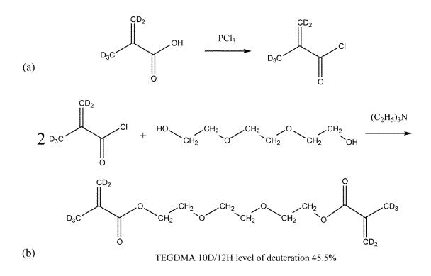
**Figure 2.1.** (a) Deuterated methacrylic acid combined with phosphorus trichloride in preparation for combining with triethylene glycol. (b) Combining deuterated methcroyl chloride with hydrogenated triethylene glycol to yield a partially deuterated TEGDMA monomer with 45.5% deuteration by molecular weight of the original hydrogen atoms.
