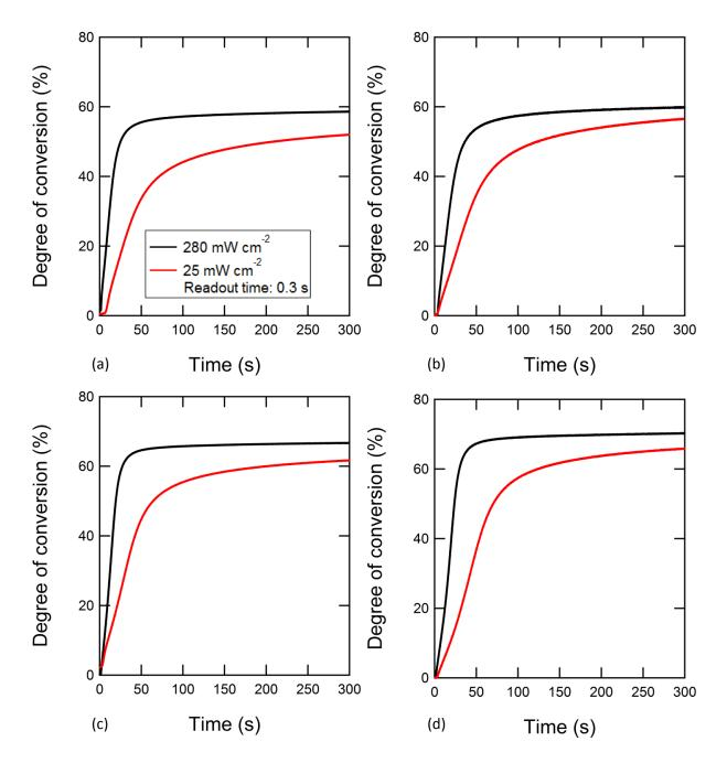
**Figure 3.7.** Degree of conversion in real time during illumination of resin samples initiated with CQ for (a) 70/30, (b) 60/40, (c) 50/50 and (d) 40/60 wt% blends. Solid black lines correspond to samples irradiated with 280 mWcm<sup>-2</sup> of light whilst the red line indicates an energy output of 25 mWcm<sup>-2</sup>.
