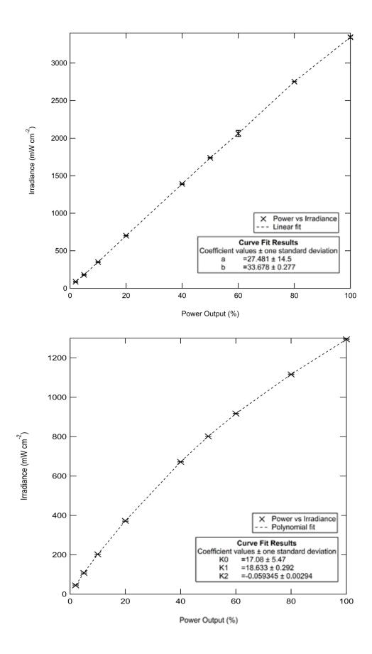
**Figure 2.4.** Calibration curves to obtain the integrated irradiance of the light engine as a function of the percentage power output for the **(top)** blue and **(bottom)** cyan colour channels. Error bars represent the standard deviation for three repeat measurements of the irradiance.
