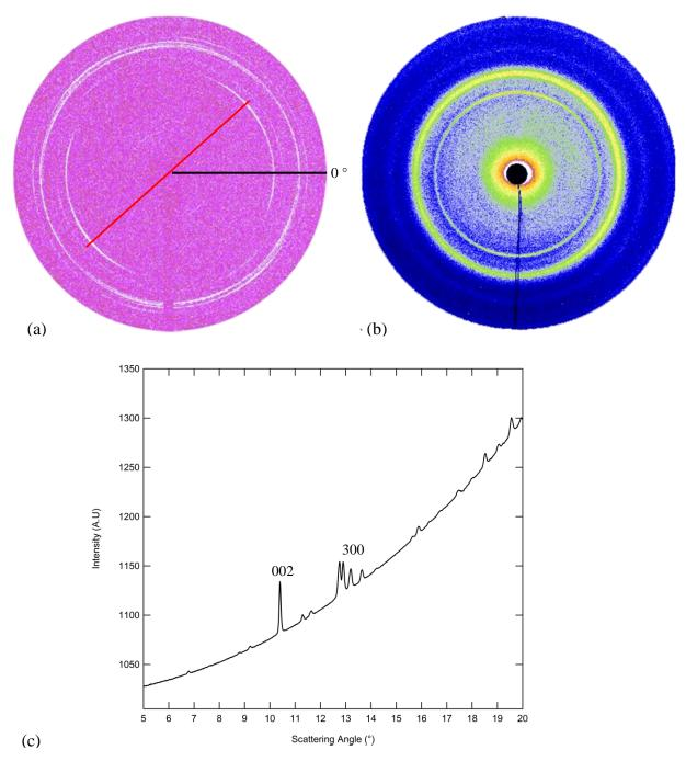
**Figure 7.2.** (a) Variation in intensity of the (002) diffraction ring is indicative of texture, whilst (b) a complete ring demonstrates little or no texture. Preferred orientation is defined from  $0^{\circ}$  which points east on the detector face, increasing azimuthally in the counter-clockwise direction. (c) A 1-D diffraction spectra with the (002) and (300) reflections corresponding to peaks located at ~  $10^{\circ}$  and ~  $14^{\circ}$  respectively.
