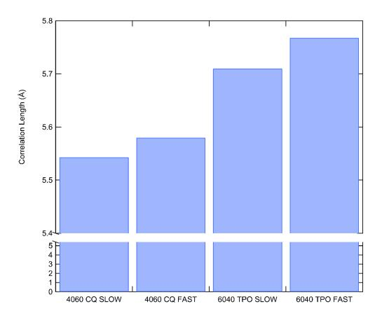
**Figure 4.8.** Final correlation lengths for peak (c)  $(q \sim 1.15 \text{ Å}^{-1})$ , for each resin formulation and irradiance protocol.
