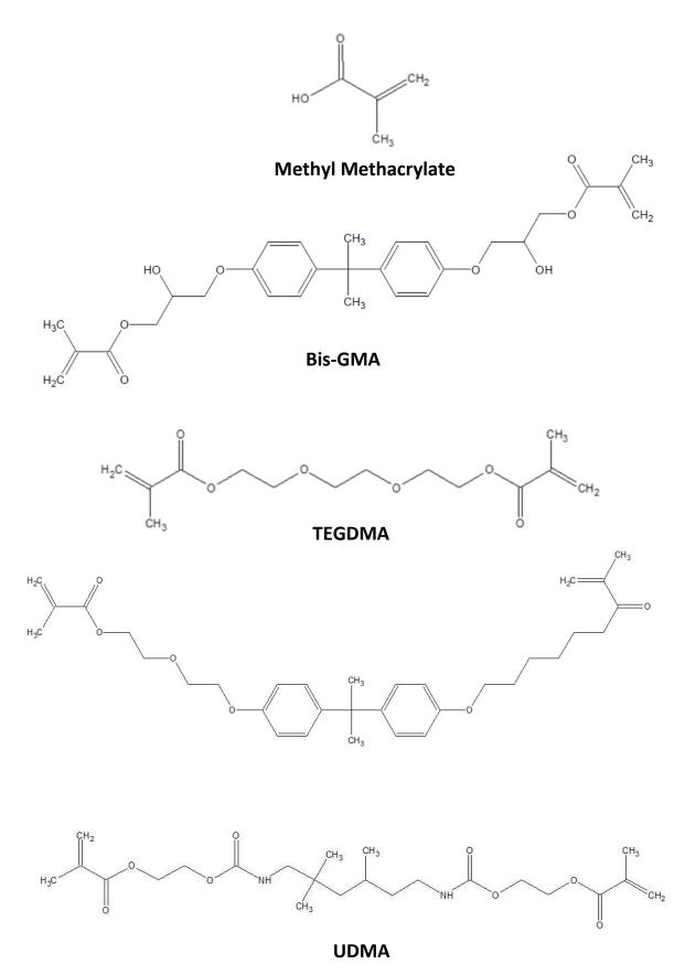
**Figure 1.3.** The chemical structure of monomers commonly used in the formulation of commercial and experimental RBCs.
