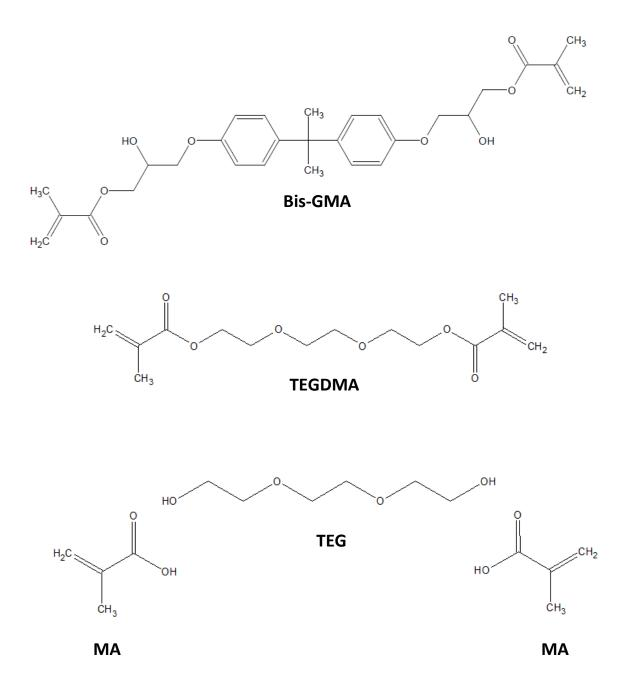
**Figure 3.3.** Chemical structures of Bis-GMA and TEGDMA monomers used to formulate each blend. Methacrylic acid (MA) and triethylene glycol (TEG) were used to simulate the chemical structure and dynamic behaviour of the TEGDMA monomer during polymerisation.
