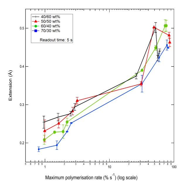
**Figure 3.12.** Maximum chain extension for each resin blend (viscosity) versus polymerisation rate (irradiance). CQ initiated resins are shown by the first four points, whilst the other data points refer to TPO initiated resins. Error bars represent uncertainty in the values as calculated by propagation of errors. Resins polymerised at higher rates display the greatest increase in the correlation length. Data was obtained from BM28 (ESRF).
