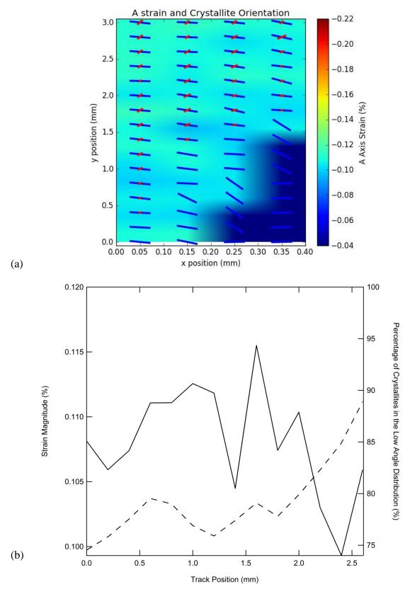
**Figure 7.9.** (a) Relative proportions of two crystallite orientations, red and blue bars, overlaid on to strain data. The aspect ratio has been altered, blurring the image, to allow for orientation bars. (b) Crystallographic strain in the a axis plotted against the proportion of crystallites in a predominantly horizontal orientation as a function of track position. Data is taken from the first track of the tooth specimen subjected to the fast polymerisation regime.
