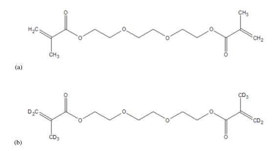
Figure 4.1. (a) Fully hydrogenated TEGDMA and (b) partially deuterated TEGDMA where the methyl and methylene groups have had hydrogen exchanged with deuterium.
