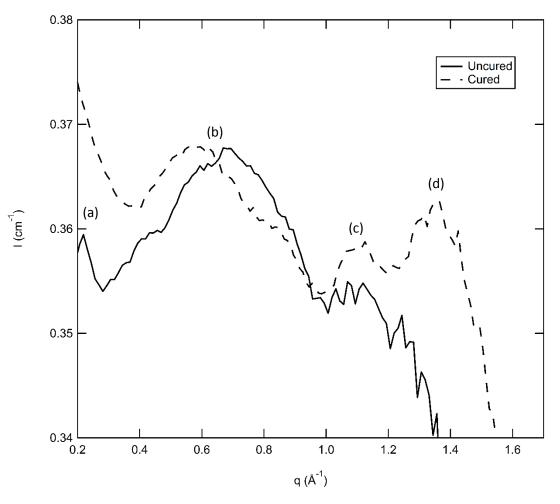
**Figure 4.2.** Small angle neutron scattering spectra of a 40/60 wt % (Bis-GMA/d-TEGDMA) blend initiated with CQ, prior to photo-polymerisation (solid line) and after photo-polymerisation (broken line). Three prominent scattering features are located at  $q \sim 0.6$ , 1.15 and 1.4 Å<sup>-1</sup>. The feature at ~ 0.2 may not represent a true structural feature and may instead be a low q artefact.
