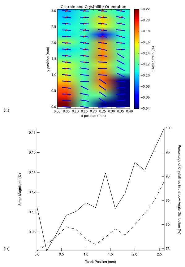
**Figure 7.8.** (a) Relative proportions of two crystallite orientations, red and blue bars, overlaid on to strain data. The aspect ratio has been altered, blurring the image, to allow for visualisation of orientation bars (b) Crystallographic strain in the c axis plotted against the percentage of crystallites in the low angle distribution as a function of track position. Data is taken from the first track of the tooth specimen subjected to the fast polymerisation regime.
