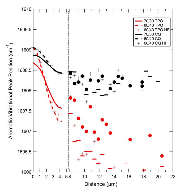
**Figure 6.5.** The aromatic wavenumber for the aromatic group at the centre of the Bis-GMA monomer is shown as a function of distance from a filler particle centre. Radially averaged wavenumber (over all particles, centre to edge) is shown to the left of the dashed line, whilst the wavenumber value at the midpoint between particle centres is shown to the right. (**inset**) The chemical structure of the Bis-GMA monomer - ring strain was detected in the aromatic core.
