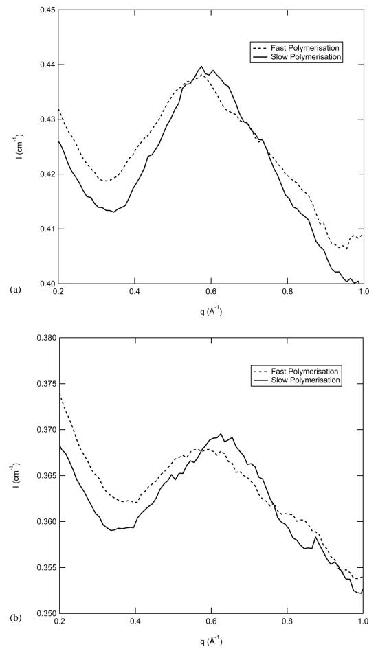
**Figure 4.6.** SANS spectra of 60/40 wt % (Bis-GMA/d-TEGDMA) blends utilising either a (a) CQ or (b) TPO photo-initiator. Resin samples polymerised at high irradiance densities are referred to as the fast regimen (broken black line) whilst low irradiance density curing protocols are termed slow regimens (solid black line).
