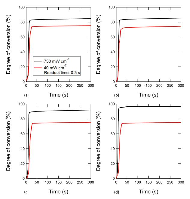
**Figure 3.10.** Real time degree of conversion during illumination of resin samples initiated with TPO for (a) 70/30, (b) 60/40, (c) 50/50 and (d) 40/60 wt% blends. Solid black lines correspond to samples irradiated with 730 mWcm<sup>-2</sup> of light whilst the red line indicates an energy output of 40 mWcm<sup>-2</sup>.
