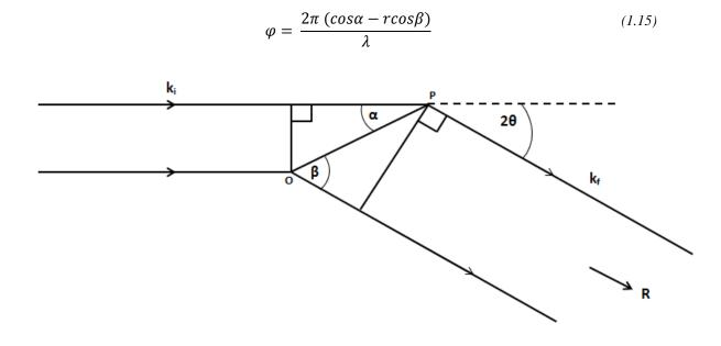
Figure 1.11. Schematic of scattering from a two atom system.
