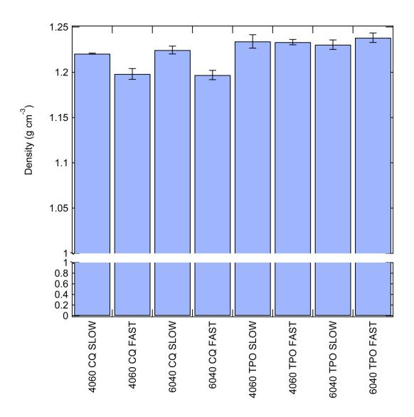
**Figure 4.10.** Density measurements of hydrogenated counterparts to deuterated resin blends used for SANS. Hydrogenated versions were used as each sample formulation could be reproduced several times to gain better statistics, unlike for deuterated samples. Error bars represent the standard deviation for three repeat measurements per sample.
