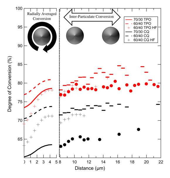
**Figure 6.3.** Degree of conversion is shown as a function of distance from a filler particle centre. Radially averaged conversion (over all particles, centre to edge) is shown to the left of the dashed line, whilst conversion at the midpoint between particle centres is shown to the right.
