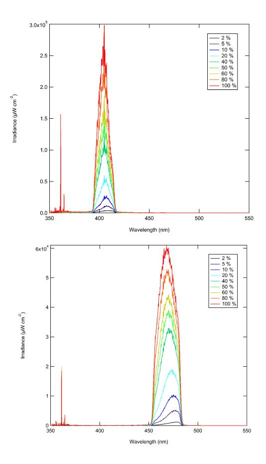
Figure 2.3. Peak emission irradiance as a function of increasing percentage power output from the light engine for the (Top) blue and (bottom) cyan colour channels.
