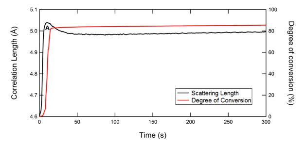
**Figure 3.11.** Real time degree of conversion (red line) and scattering length (black line) for a 60/40 wt% blend initiated with TPO. Auto-acceleration in the resin bulk corresponds to a large initial increase in the correlation length. The point of auto-deceleration in the polymer network (the start of the plateau in the *DC* plot) coincides with the maximum increase in scattering length.
