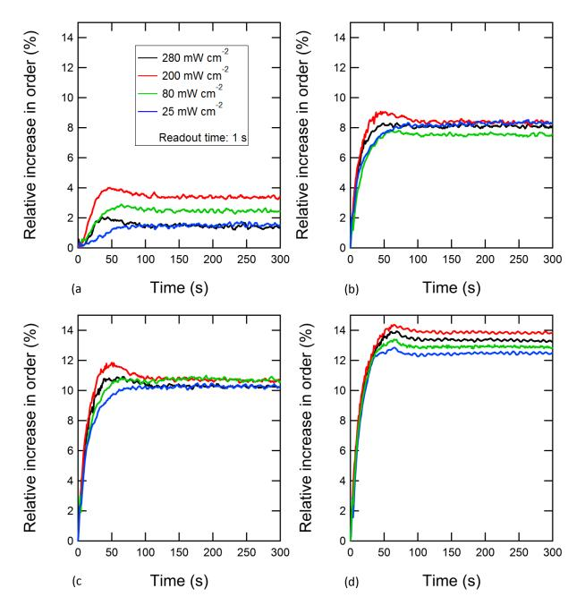
**Figure 3.6.** The relative percentage increase in short range order during photo-polymerisation as a function of polymerisation rate for resin samples initiated with CQ for (a) 70/30, (b) 60/40, (c) 50/50 and (d) 40/60 wt% blends. Changes in order are similar and occur simultaneously to those observed in the correlation length for CQ initiated blends.
