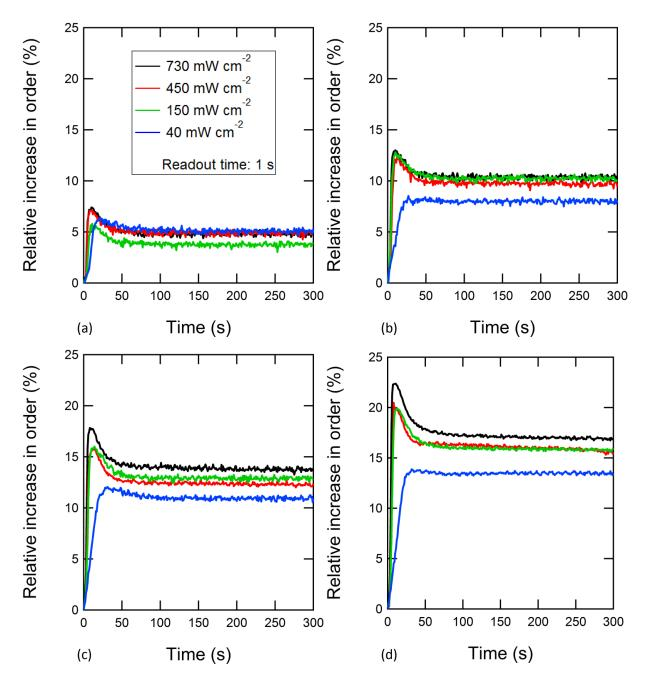
**Figure 3.9.** Changes in the relative order throughout photo-polymerisation for TPO initiated (**a**) 70/30, (**b**) 60/40, (**c**) 50/50 and (**d**) 40/60 wt% resin blends. Unlike CQ initiated resins, these systems demonstrate a large relaxation feature.
