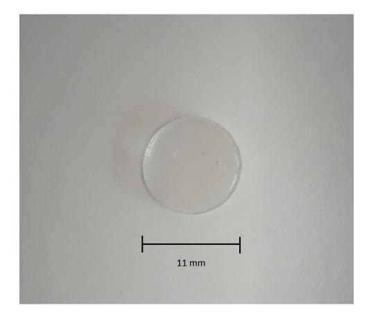
Figure 2.6. An unfilled resin disc test specimen.
