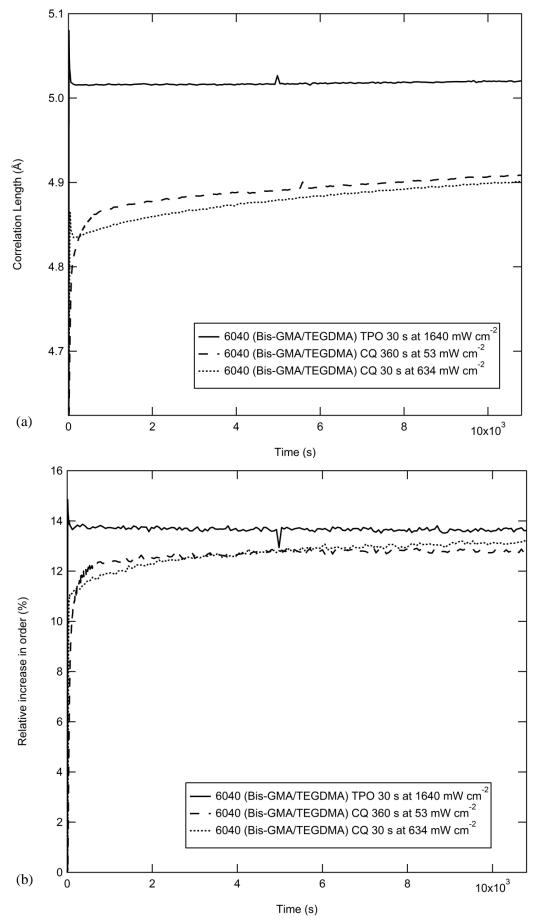
**Figure 4.11.** Real time evolution of the (**a**) correlation length and (**b**) relative increase in order for 60/40 wt% (Bis-GMA/TEGDMA) blends. Resins photo-initiated with CQ at high (dotted line) and low (broken line) light irradiance densities are shown in addition to a TPO initiated resin polymerised at a relatively high light irradiance density (solid line)
