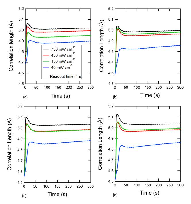
**Figure 3.8.** Time resolved changes in the correlation length as observed in TPO initiated resins for (a) 70/30, (b) 60/40, (c) 50/50 and (d) 40/60 wt% blends (Bis-GMA/TEGDMA) during 300s of photopolymerisation for a range of reaction rates. Initial increases in the correlation length upon illumination and subsequent relaxations are larger and more rapid for TPO initiated resins, corresponding to a faster polymerisation rate.
