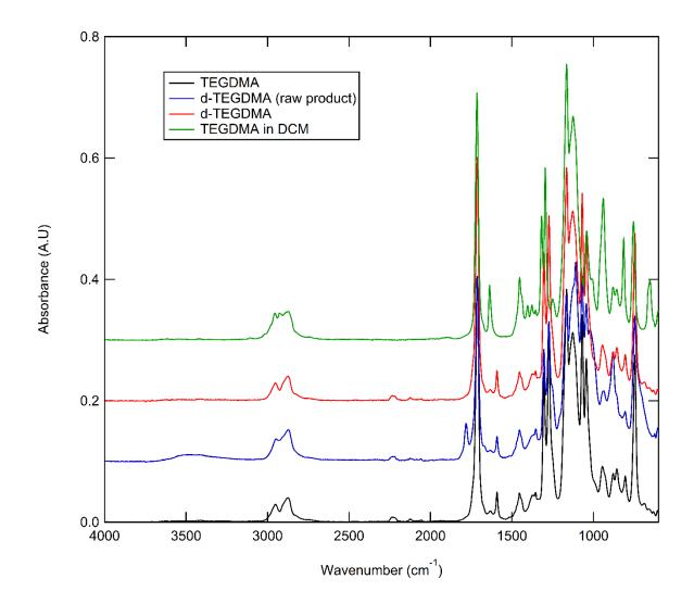
**Figure 2.2.** FTIR spectra for deuterated undeuterated variants of the TEGDMA monomer. Spectra for the d-TEGDMA at specific steps of purification are also shown and are offset in the absorbance axis for clarity.
