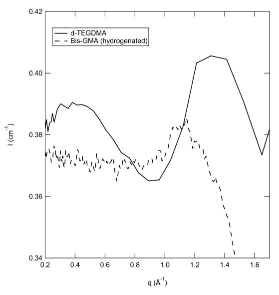
Figure 4.3. SANS spectra of liquid monomers d-TEGDMA (solid black line) and hydrogenated Bis-GMA (broken black line).
