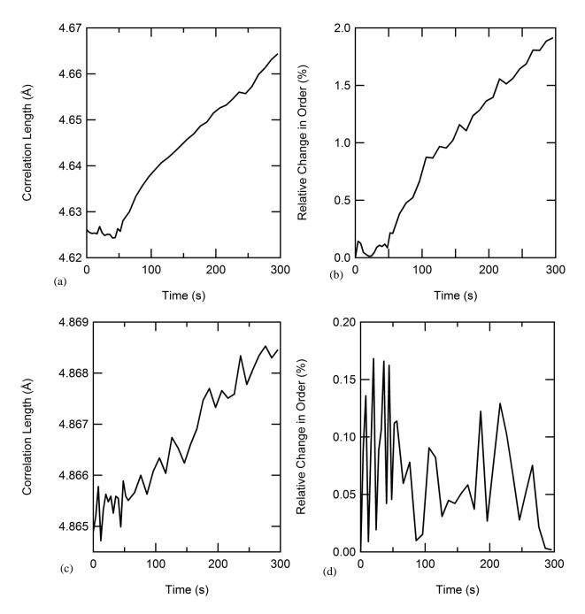
**Figure 10.1.** Real time evolution of the correlation length reported in chapter three when exposed to X-rays for a 60/40 wt% (Bis-GMA/TEGDMA) sample with TPO photo-initiator in the (a) liquid monomer and (c) solid polymer form. Analogous plot for changes in short range order are shown in (b) and (d).
