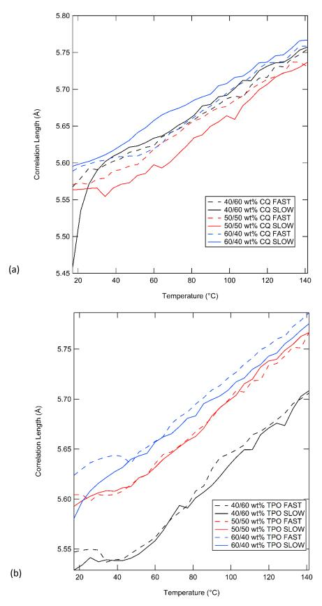
Figure 5.3. Correlation length as a function of temperature for (a) CQ and (b) TPO initiated RBCs.
