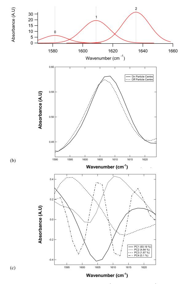
**Figure 6.4.** (a) Deconvolution of the aromatic  $(1609 \text{ cm}^{-1})$  and aliphatic  $(1637 \text{ cm}^{-1})$  absorption bands. (b) The aromatic absorption band taken as a line transect from the centre of a particle into the resin matrix. (c) Loading vectors of the aromatic peak over the aforementioned line transect.
