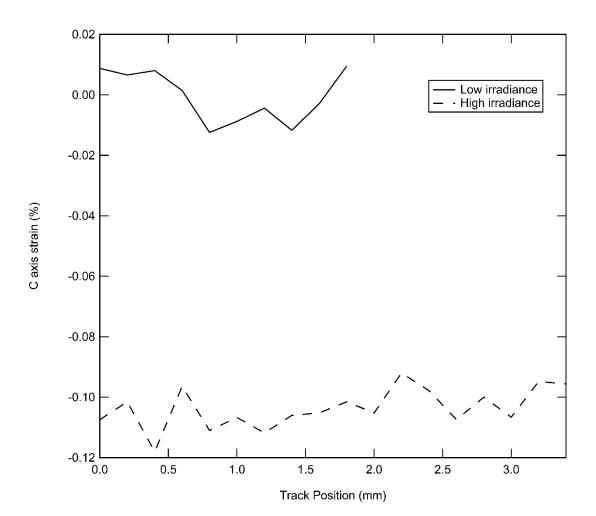
**Figure 7.5.** The percentage change in the c axis length, following the application of an RBC, is shown as a function of the measurement position along (here the top of the track position starts at 0 mm) the respective track for fast (broken line) or slow (solid line) polymerisation regimes.
