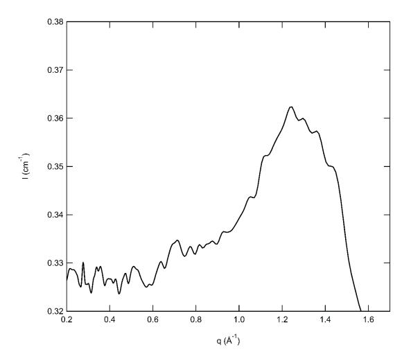
**Figure 4.4.** SANS spectra of a completely hydrogenated 60/40 wt% (Bis-GMA/TEGDMA) sample with a CQ initiator system.
