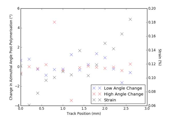
**Figure 7.7.** Changes in crystallite orientation angle post polymerisation for high irradiance curing, for the low (black solid line) and high (black broken line) angle directions, plotted as a function of track position with strain in the c lattice overlaid (red line). Track position is defined as 0 mm equal to the top of the tooth fin track and 2.4 mm representing the bottom of the fin.
