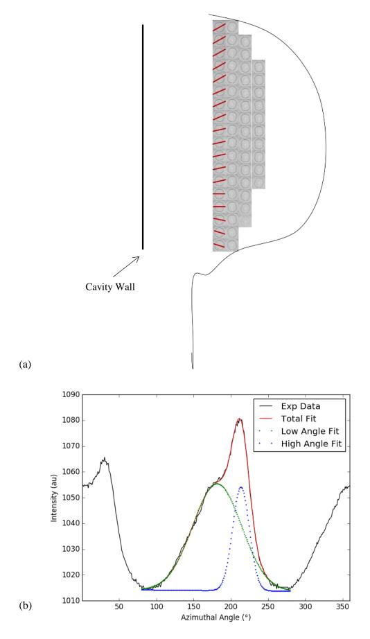
**Figure 7.3.** (a) A composite image showing individual 2-D diffraction spectra, for each measurement along a track, superimposed on to a schematic of a tooth fin. Bisection of the (002) diffraction ring through points of greatest intensity yields the approximate direction of preferred orientation, which is shown as a red line. (b) Azimuthal integration of the (002) diffraction ring shows that two directions of crystallite/prismatic orientation exist within the tooth enamel.
