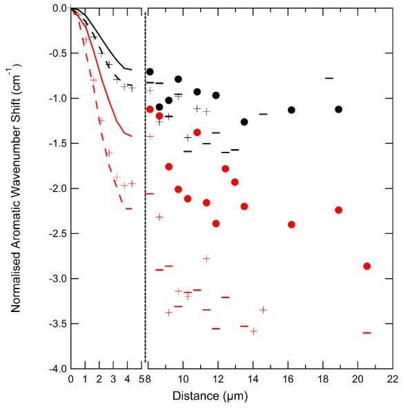
**Figure 6.7.** The decrease in the aromatic wavenumber (an increase in residual strain), normalised to the degree of conversion at each distance increment. The generation of residual strain within the RBC is ranked by the relative differences in polymerisation rate.
