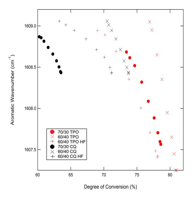
**Figure 6.6.** The radially averaged decrease in the aromatic wavenumber as a function of monomer to polymer conversion. Each plotting point represents a distance increment of 0.54  $\mu$ m from the centre of the filler particle, the first point to the left, to the edge of the particle. Here data are replotted with different symbols to previous figures to clarify the number and location of points.
