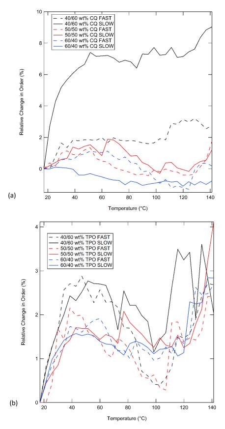
Figure 5.4. Relative changes in order as a function of temperature for (a) CQ and (b) TPO initiated RBCs.
