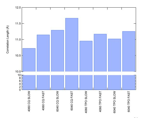
**Figure 4.5.** Correlation lengths, corresponding to the scattering peak initially located at  $q \sim 0.6 \text{ Å}^{-1}$ , post photo-polymerisation for the respective resin blend test specimens.
