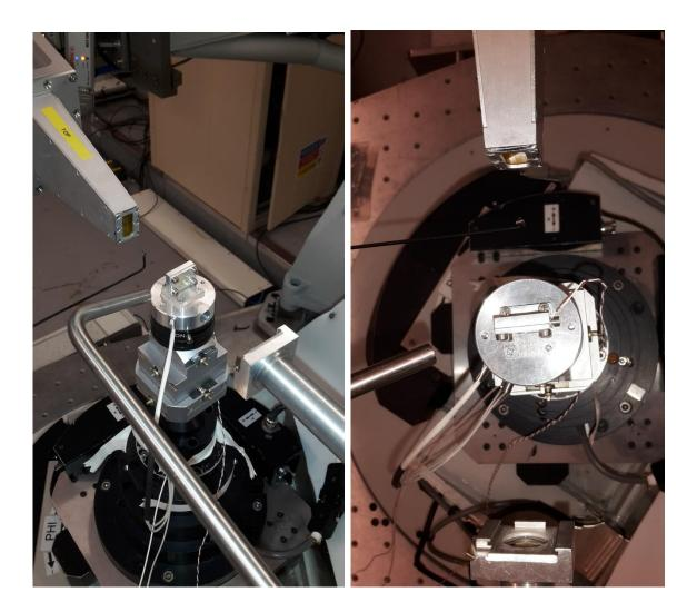
**Figure 5.1.** (left) Two Aluminium plates, mounted onto a heated kinematic stage, heats a resin disc test specimen held between the plates. X-rays impinge normal to the sample face and scatter into a Pilatus 100 K detector mounted onto a 2 $\theta$  detector arm. (**right**) Top down view of the experimental set-up. The pipe to the left of the image blows cold air (20 °C ± 1 °C) to cool the stage after heating.
