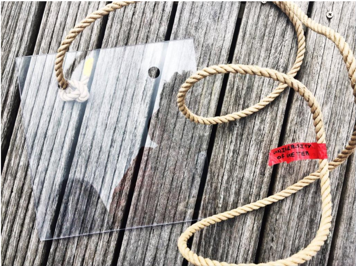
Figure 4.1: Settlement plate before being placed in Milbay Marina (Photograph provided by A. Porter).
