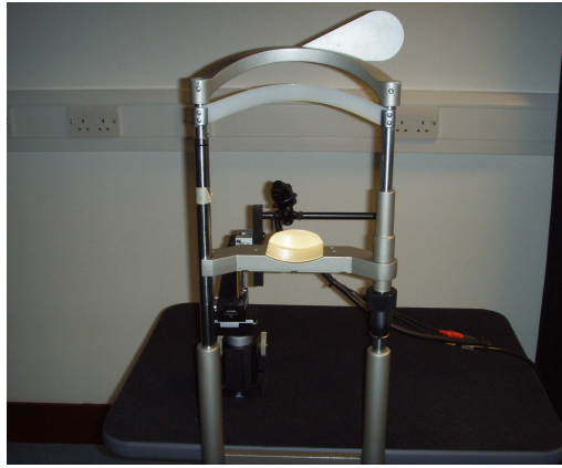
Figure 2.1: Set-up for testing of subjects. Video eye-tracker indicates the position of the pupil as required for paracentral measurements.
