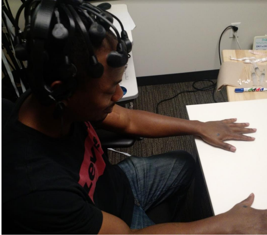
Figure 2: Subject awaiting pressure stimulus test. Dry quick-20 EEG device is connected in testing room; with hands (adductor pollicis) marked using dry erase marker for points of stimulus and with Quick-20 Dry EEG connected to detect brain waves.
