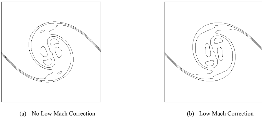
Figure 5: Passive Scalar iso-lines of the final vortex structure produced at time t = 6.0 s from the CNS3D-FV-M3 scheme on a 64 \times 64 grid with Mach number M = 0.2 .
