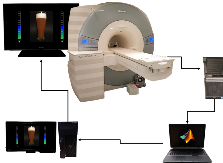
Fig. 2 Real-time fMRI neurofeedback setup. Acquired images are reconstructed and send to a laptop running in-house MATLAB (MathWorks Inc., Sherborn, MA, USA) scripts based on SPM8 (Wellcome Department of Cognitive Neurology, London, UK) functions to preprocess the images and extract the neurofeedback signal. The feedback value is send to a computer running Presentation software (Neurobehavioral Systems, Inc., Albany, CA, USA) and presented to the participant in the scanner as a thermometer value besides a picture of an alcoholic beverage
