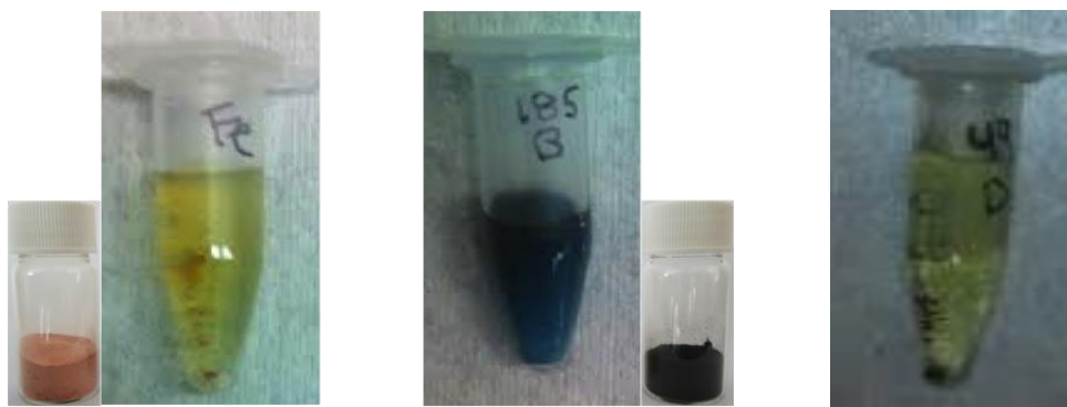
Figure S12 | Prussian blue test of Fe-BTC (left) and Fe-BTC/PDA-19 (middle) and Fe-BTC/PDA-19 soaked in a Hg solution (right). The change in color from yellow to blue illustrates free catechols throughout the composite.
