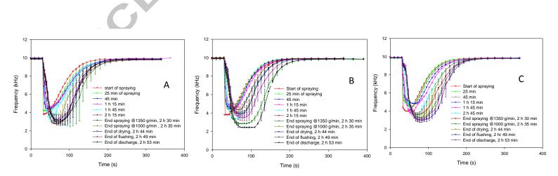
Figure 2: BARDS dissolution profiles of pellet samples from the sub-coating process for three individual batches of Omeprazole pellets, A, B and C. 300 mg of pellets were dissolved in 0.01 M NaOH for each experiment. All profiles were measured in duplicate.
