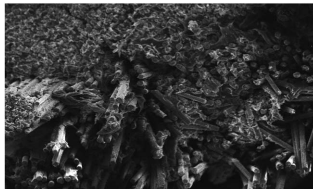
FIG. 5. SEM image of a fractured Pultrusion specimen ( \times 250 ).
