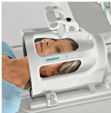
Figure 1.4: An 8-channel RF coil for clinical brain imaging (Source: Siemens [2]).
