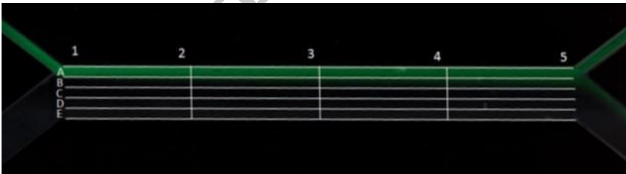
Fig. 3. Mesh sketch for image analysis and its application in an experimental image with the asymmetric chip (configuration 1).
