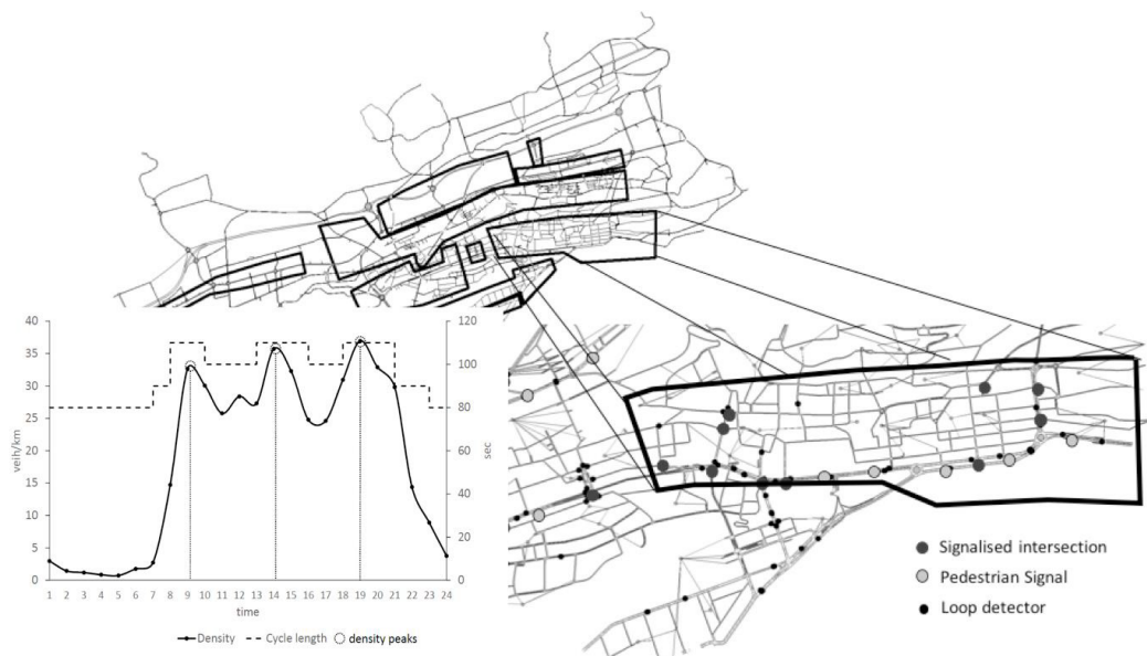
Fig 1- Road network of Santander: main sub-areas with traffic light controls and a focus on the examined zone
