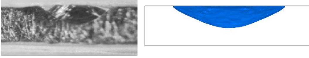
FIG. 6.8 – Comparison between visualizations of Yang et al. (2004) and present simulation with the JADIM code with \theta_{GDL} = 120^\circ and \theta_W = 30^\circ .
