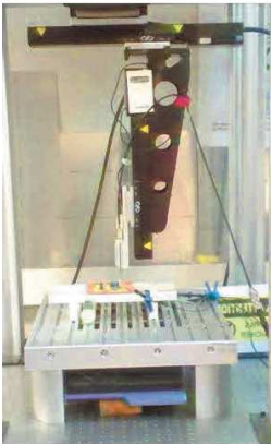
3D Motorized support res. xyz 10µm
