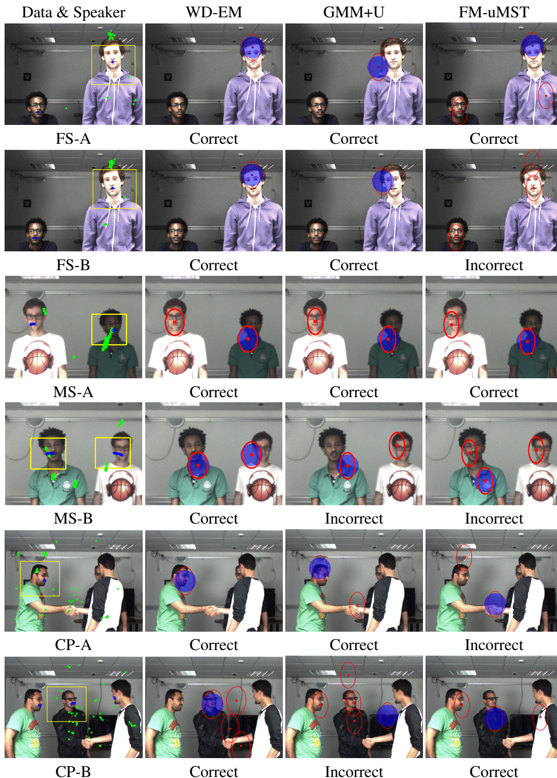
Figure 4.4: Results obtained on the fake speaker (FS), moving speaker (MS) and cocktail party (CP) sequences. The first column shows the audio (green) and visual (blue) observations, as well as a yellow bounding box that shows the ground-truth active speaker. The second, third and fourth columns show the mixture components obtained with the WD-EM, GMM+U and FM-uMST methods, respectively. The blue disks mark components that correspond to correct detections of active speakers, namely whenever there is an overlap between a component and the ground-truth bounding box.
