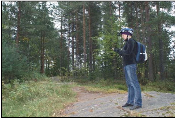
Figure 1. The goals of the test tasks were to resolve the current location on the mobile map and to navigate to a predefined position. The eye-tracking camera was attached on the bicycle helmet and the laptop used for data recording was carried in the backpack.
