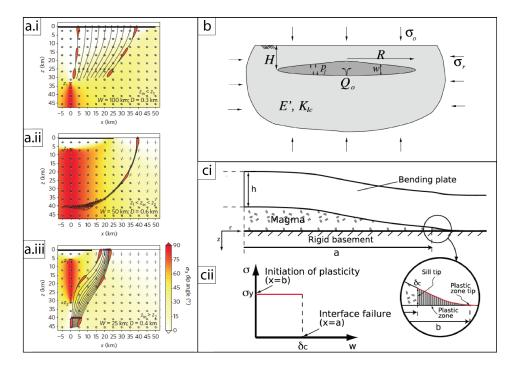
1910 Figure 9: Example numerical models of sheet intrusions: a) dyke trajectories in the presence1911 of a stress barrier (Maccaferri et al. 2014), b) the growth of a laccolith (Bunger and Cruden
