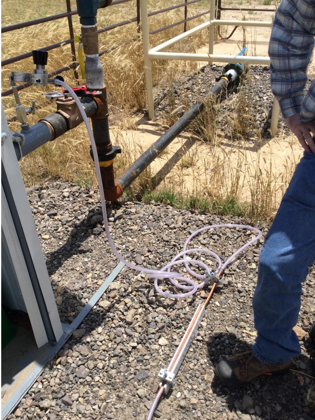
Figure 2.1.: Collection of natural gas samples from the Bonnie Carson #1 well using the field sampling setup outlined above, Ford County, Kansas in 2014.
