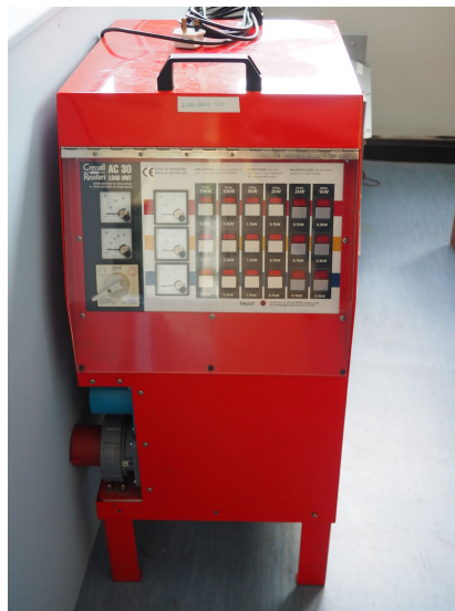
Figure 4.13: Photograph of resistor bank.
