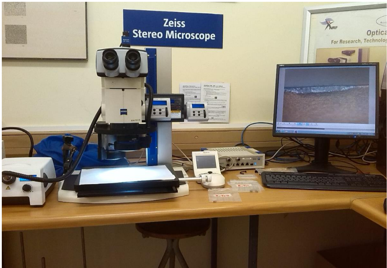
Figure 4-9: ZEISS light microscope with image analyzer
