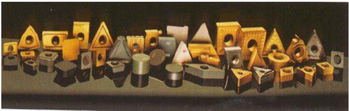
Figure 2-13: Typical insert shapes and Tip angles [44]
