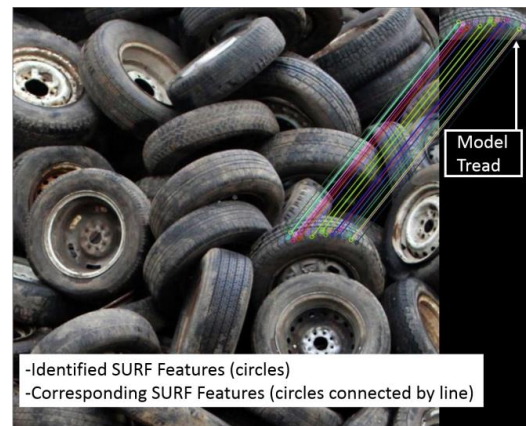
Figure 3 - SURF Feature Matching between image of stockpile containing multiple tyres and single tyre example manually extracted from the image.
