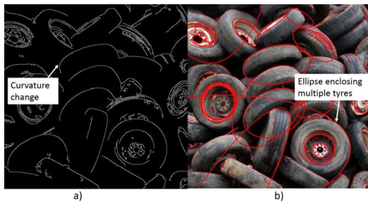
Figure 1 - Pre-processed edge image (a). Detected ellipses and circles drawn on original image (b).
