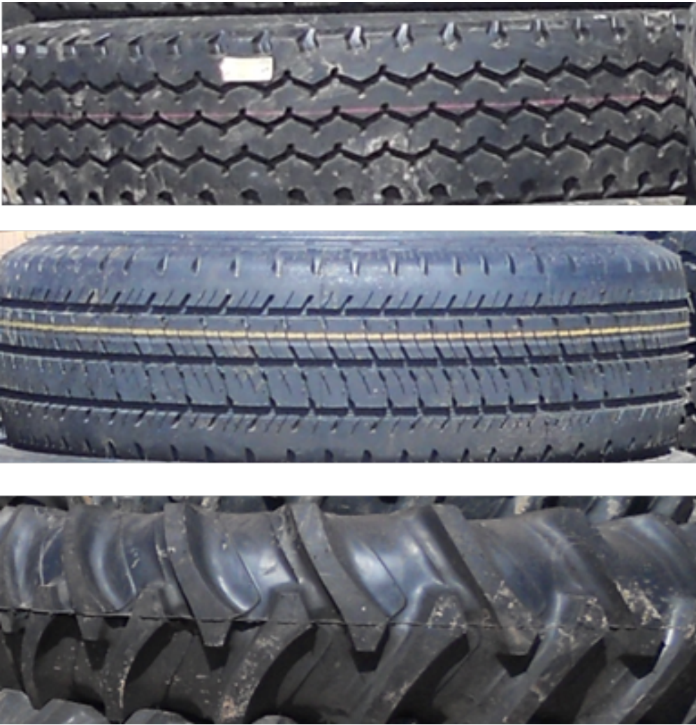
Figure 2: Subset of images (truck, passenger, 4x4) used in general level categorization of tyres.
