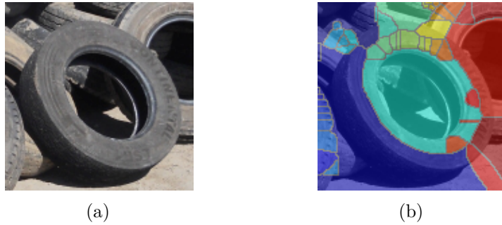
Figure 2.12: Application of watershed algorithm to image of a tyre.
