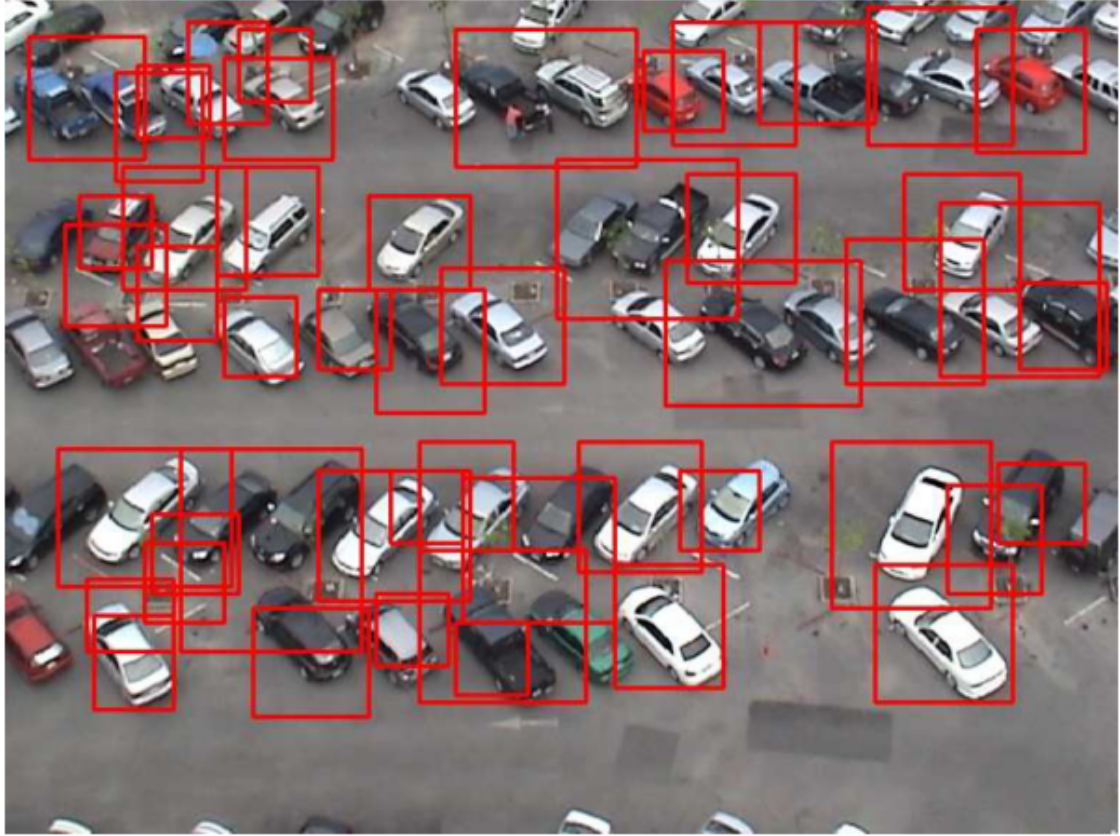
Figure 3.15: Visualization of detections for a vehicle counting method Tongphu et al. (2009).
