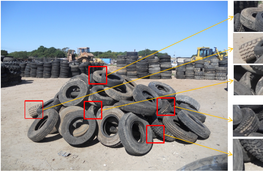
Figure 4.1: Features from single image matched to subregion of a tyre stockpile image.
