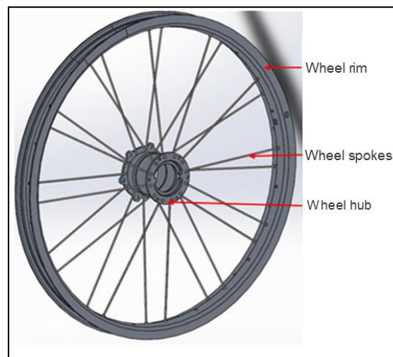
Figure 23- Computational FEA model of commercial wheel ( Dassault Systèmes SolidWorks )
