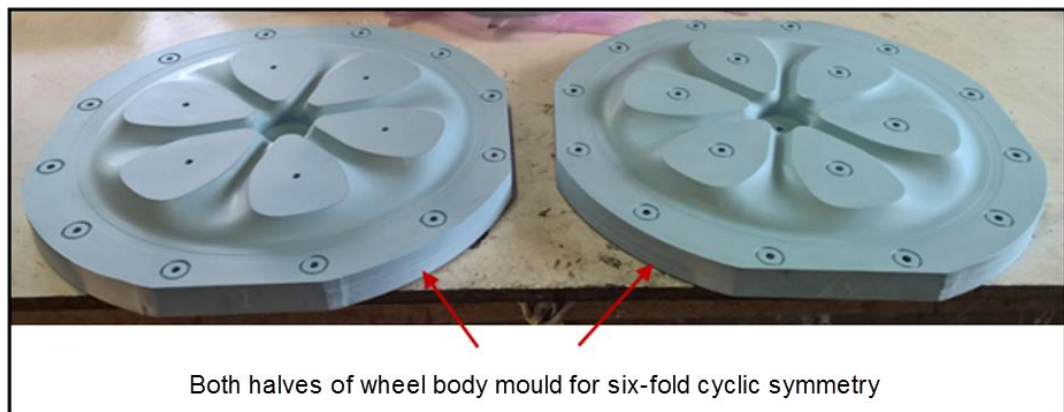
Figure 42 - Both halves of wheel body mould before layup or assembly
