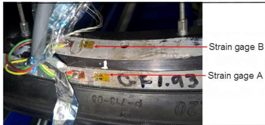
Figure 17 - Uniaxial strain gages applied to the rim of a commercial wheel
