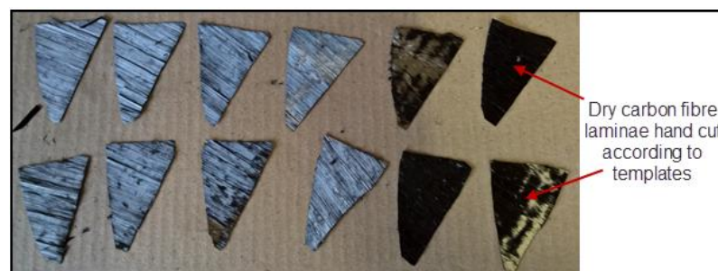
Figure 41 – Example of some of the dry carbon fibre laminae hand-cut according to the optimized composite wheel design containing refined lamina geometries
