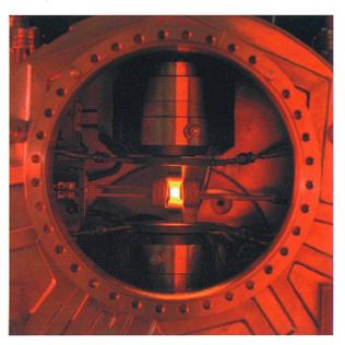
Detail of specimen mounted in vacuum chamber for thermomechanical fatique testing.
