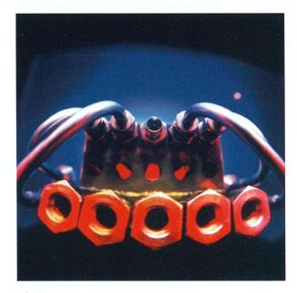
Mock-up Ds/Cn-I. Bottom-view with cooling tubes.
