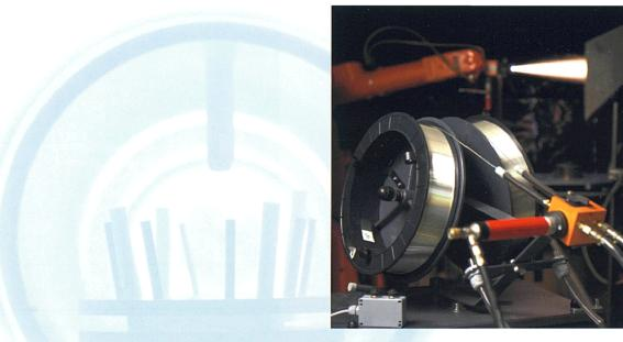
Robotized wire spraying unit, used for the deposition of thick metal coatings.
