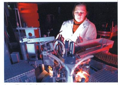
Automated filling and sealing of ampoules.
