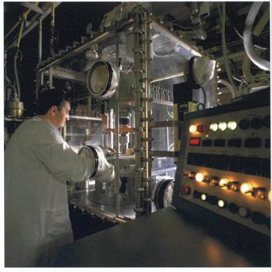
Fabrication of inert matrices (spinel MgAl<sub>2</sub>O<sub>4</sub>, zircon ZrSiO<sub>4</sub>, etc.) to replace U-238 in nuclear fuels for transmutation of the minor actinides Am and No.
