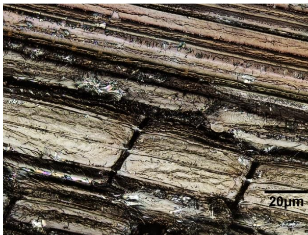
Fig. 2. 3D laser scanning confocal microscope image of a cellulosic fibrovascular bundle structure and parenchymal cells after SHS treatment at 210 °C for 3 h. Magnification: \times 1000 . Bar 20 \mu\text{m}
