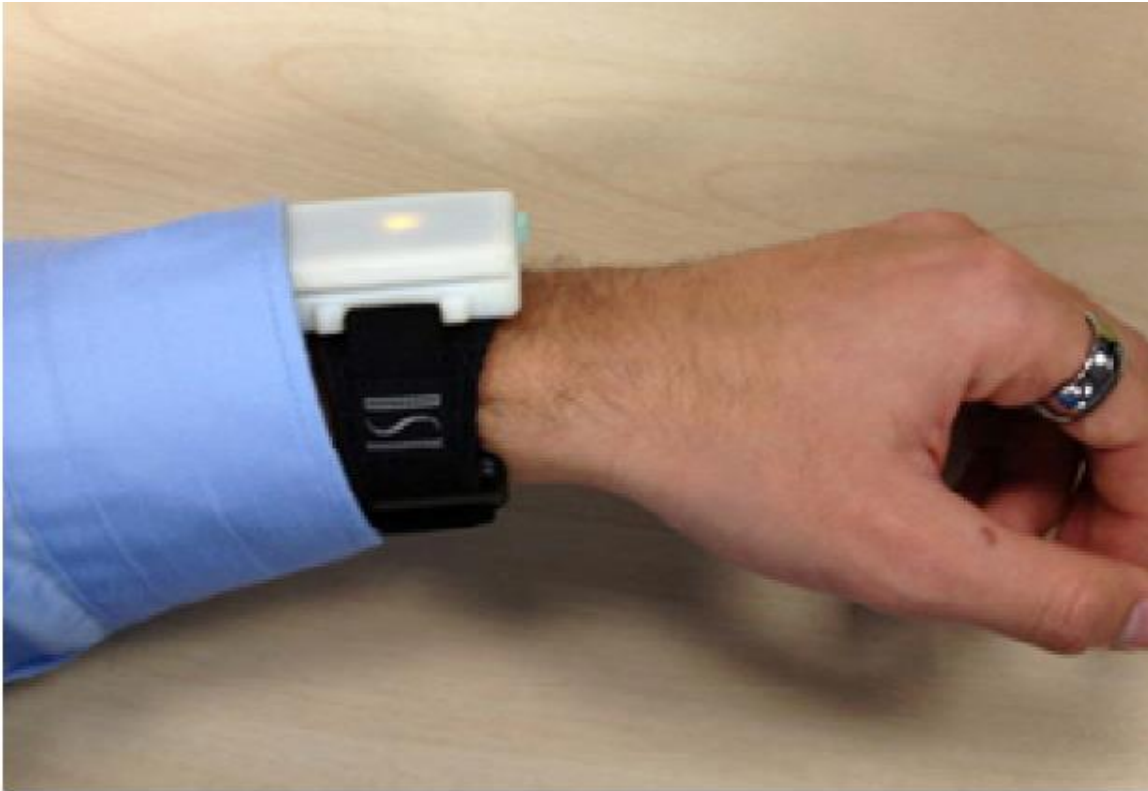
Figure 2-2: Magnetic Sensing System. Reproduced from [41]
