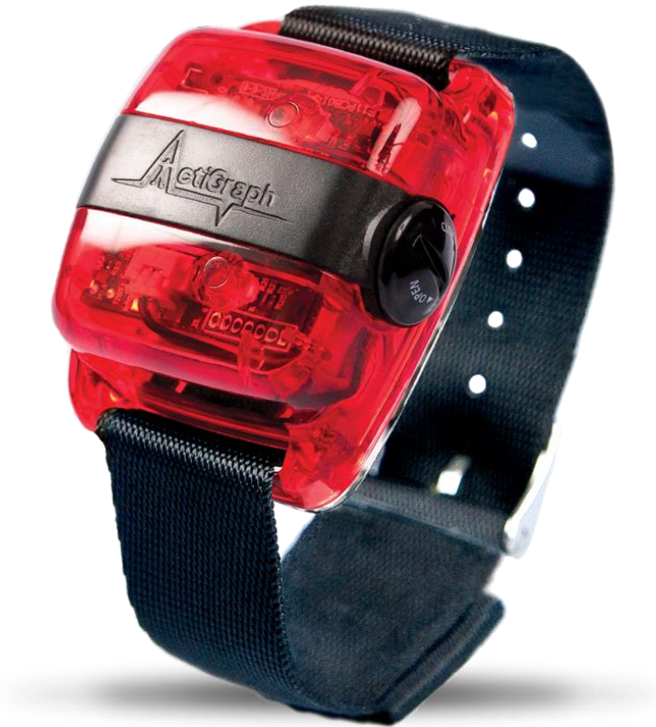
Figure 2-1: Commercially Available Inertial Sensing Based Activity Tracker. Reproduced from [38]
