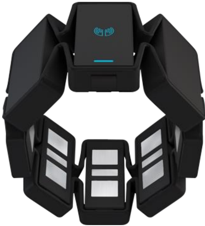
Figure 2-4: Commercially Available SEMG Arm Band. Reproduced from [49]
