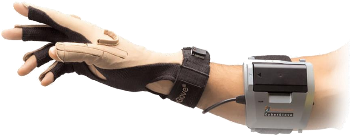
Figure 2-3: Commercially Available Sensing Glove. Reproduced from [42]
