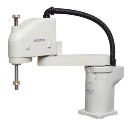
Figure 2-11 A serial SCARA robot from Mitsubishi Electric (courtesy of Mitsubishi Electric)
