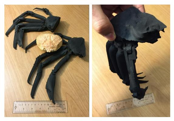
Figure 3-10 The fully articulated snow crab produced by SLS
