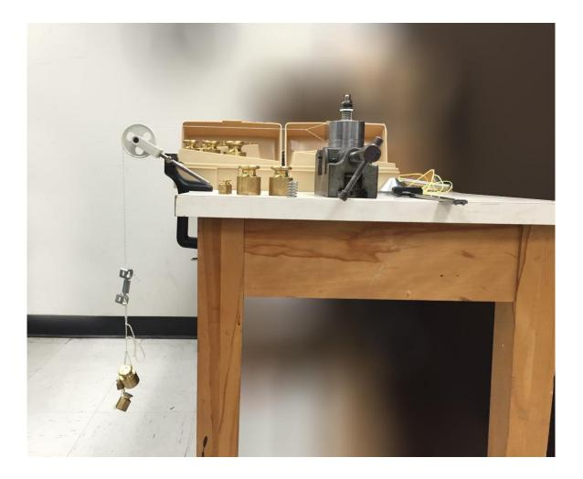
Figure 6-6 The bed test structure and the position of the parts from front view
