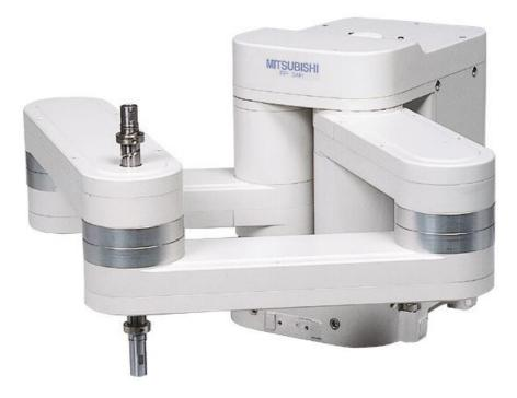
Figure 2-12 A parallel Five-Bar robot from Mitsubishi Electric (courtesy of Mitsubishi Electric)
