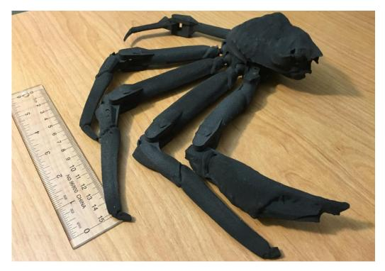
Figure 3-11 The fully articulated snow crab produced by SLS (the scale factor 1:1)
