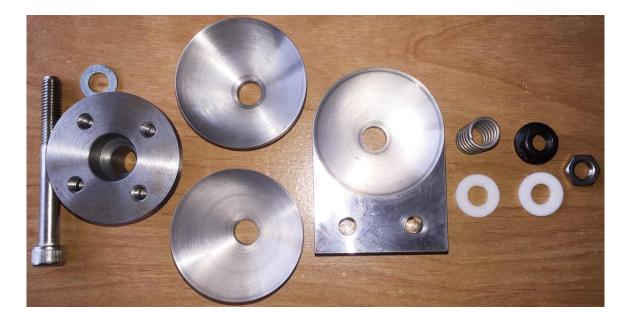
Figure 5-2 The conical joint parts
