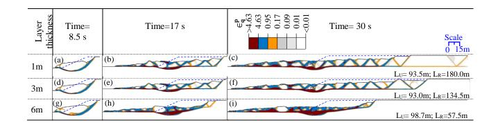
Figure 4.14: Slope-IV: Effect of change in quick clay layer thickness
