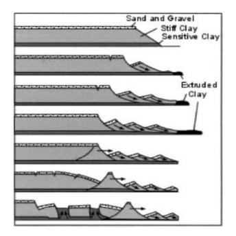
Figure 2.1: Typical failure in model test slopes for Turnagain Heights landslide
