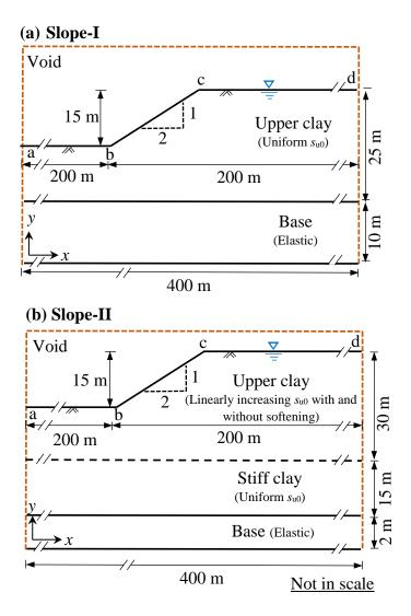
Figure 3.1: Geometry of the slopes used in FE modeling
