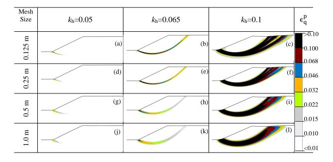
Figure 3.5: Mesh size effects on FE results based on pseudostatic analyses in Slope-II.
