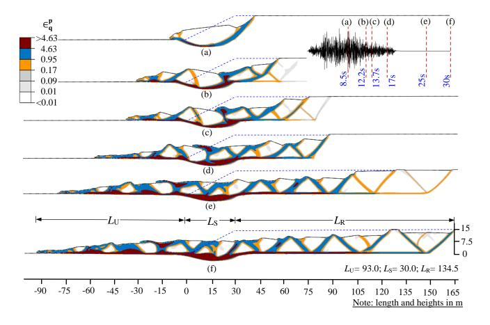
Figure 4.13: Slope-IV: Development of failure surfaces
