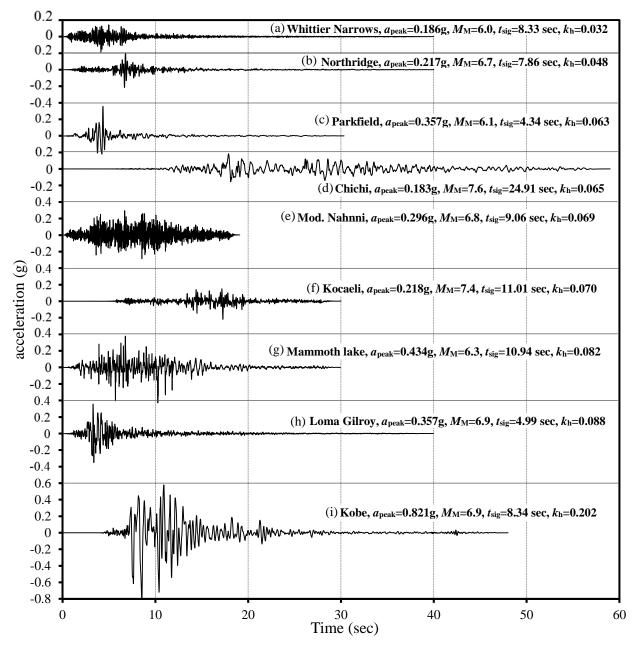
Figure 3.7: Acceleration time histories as reference earthquake input motions
