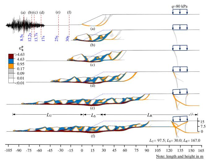
Figure 4.11: Slope-III: Development of failure surfaces
