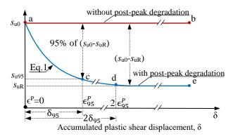
Figure 3.6: Stress strain behaviour used in FE modeling
