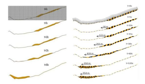
**Figure 2.3:** Progression of landslide: (left) CEL and (right) MPM (after Moormann and Hamad, 2015)
