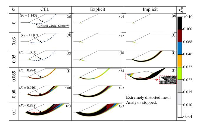
Figure 3.4: Pseudostatic analyses for Slope-II using three FE modeling approaches
