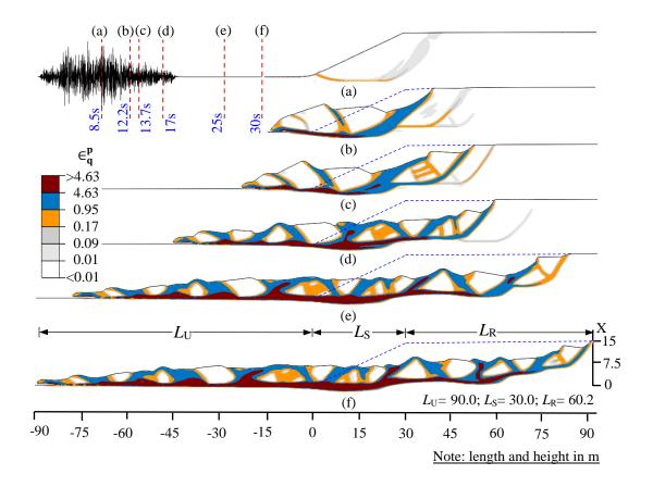
Figure 4.4: Slope-I: Development of failure surfaces
