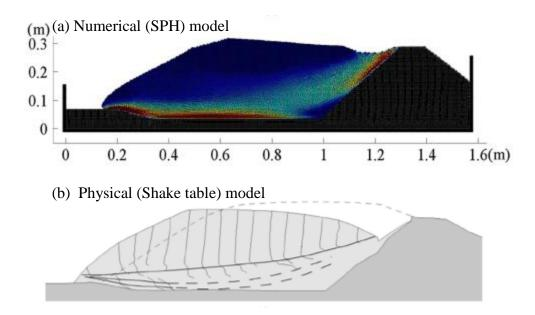
**Figure 2.2:** Comparison of simulated failure surface and deformed shape with shake table model slope test by Wartman (2005) (after Chen and Qiu, 2014).
