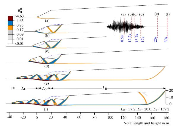
Figure 4.9: Slope-II: Development of failure surfaces
