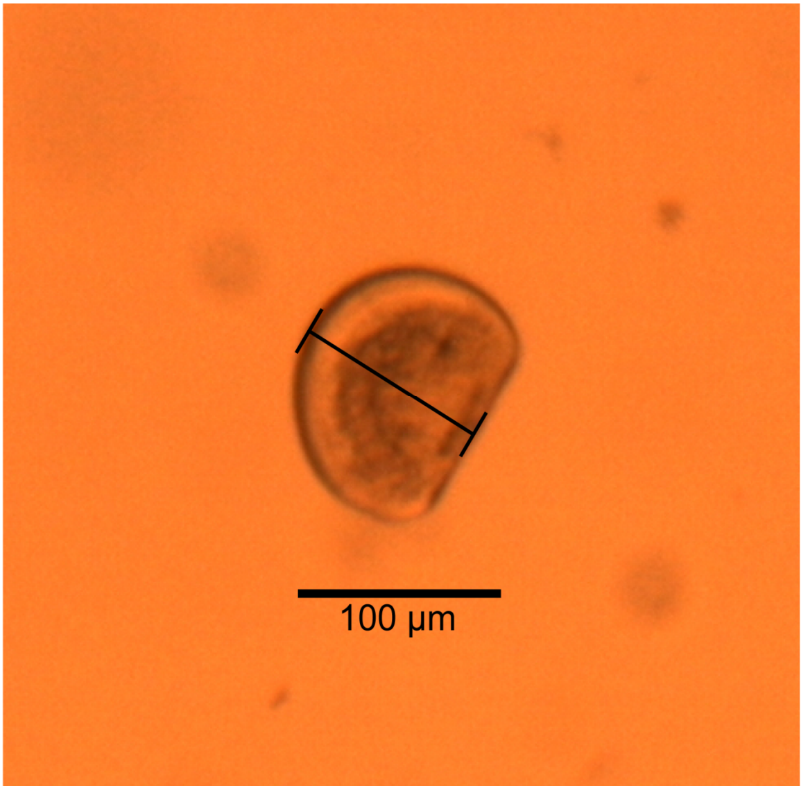
Figure 4.3. Example of typical D-stage scallop larval image indicating appropriate scale and shell height measurement.
