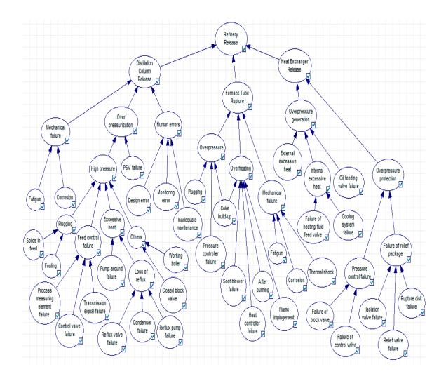
Figure 43. Bayesian network of oil release in refinery
