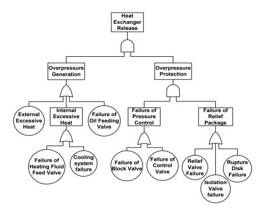
Figure 42. Fault tree for heat exchanger explosion
