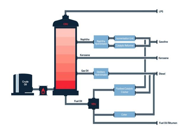
Figure 14. A schematic diagram of a typical refinery process (www.varoenergy.com)
