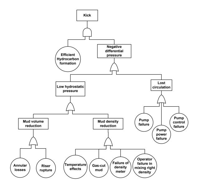
Figure 15. Fault tree analysis of offshore drilling
