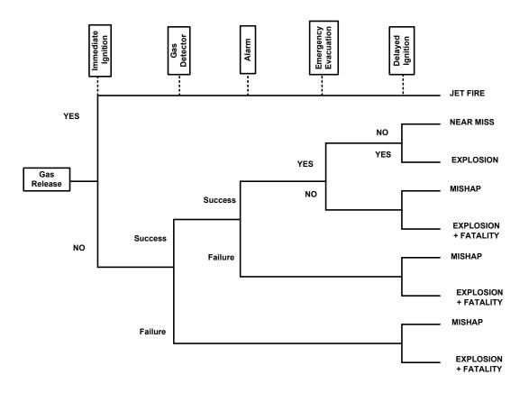
Figure 23. Event tree of gas release in liquefaction facility
