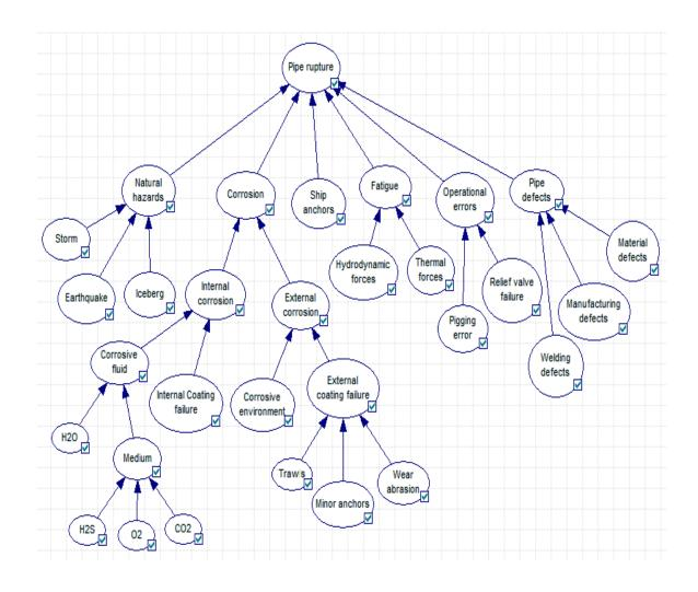
Figure 19. BN of sub-sea pipe rupture
