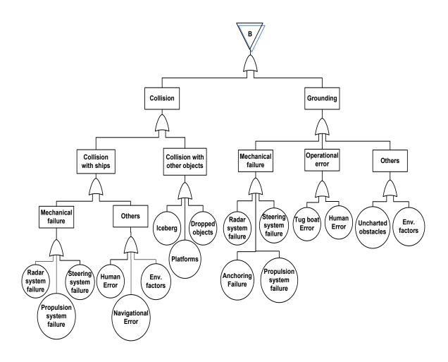
Figure 29. Fault tree for LNG release during shipping (Part B)
