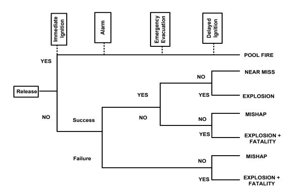
Figure 44. Event tree analysis of oil release in refinery
