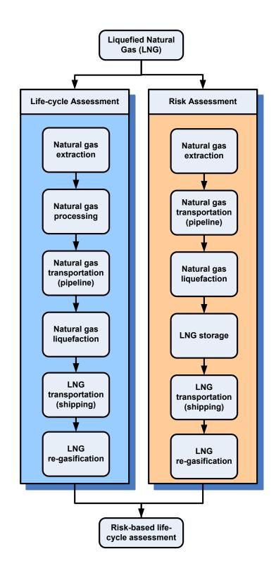
Figure 7. Risk-based life-cycle assessment of liquefied natural gas (LNG)
