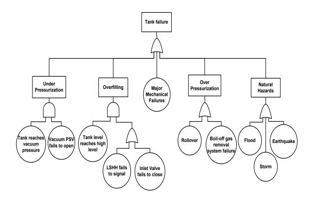
Figure 24. Fault tree of gas release from LNG storage tank
