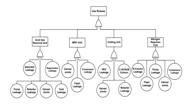
Figure 21. Fault tree of gas release in the liquefaction facility
