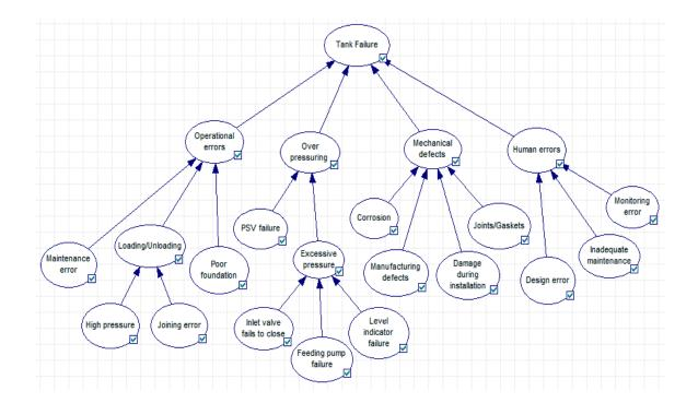
Figure 39. Bayesian network of oil release from oil storage tank
