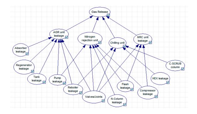
Figure 22. Bayesian network of gas release in the liquefaction facility
