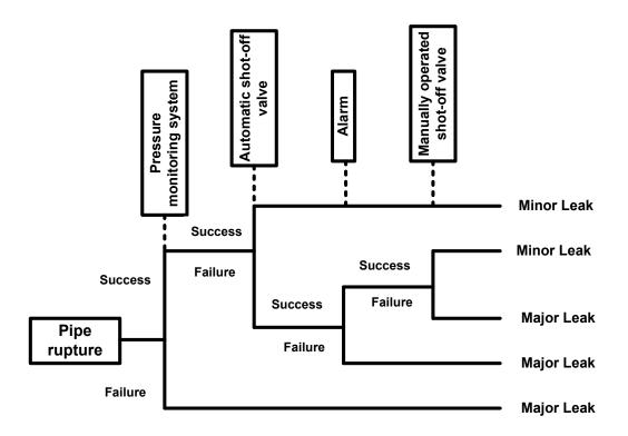
Figure 20. Event tree of sub-sea pipe rupture
