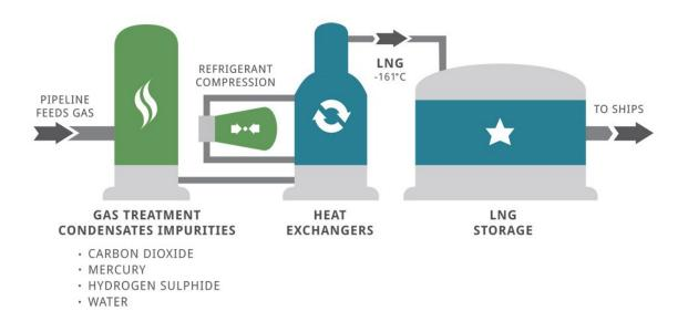
Figure 10. Schematic of liquefaction facility at Goldboro Plant (www.goldborolng.com)
