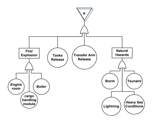
Figure 34. Fault tree for crude oil release during shipping (Part A)
