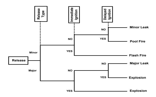
Figure 37. Event tree analysis of crude oil release during shipping
