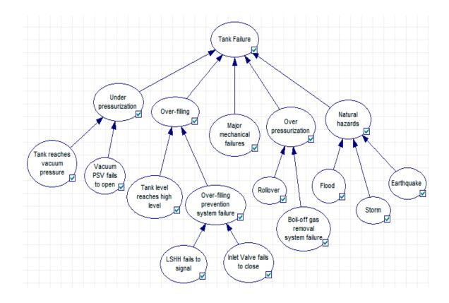
Figure 25. Bayesian network of gas release from LNG storage tank
