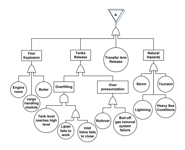
Figure 28. Fault tree for LNG release during shipping (Part A)
