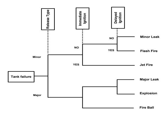
Figure 26. Event tree of gas release in LNG storage tank
