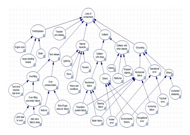
Figure 30. Bayesian network for LNG release during shipping
