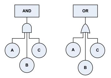
Figure 2. AND gate (left) and OR gate (right) in fault trees
