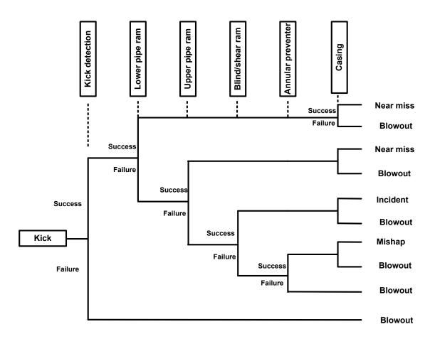
Figure 17. Event tree analysis of offshore drilling
