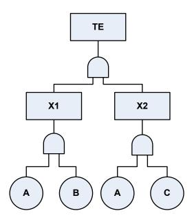
Figure 3. A fault tree with common-cause failure A.
