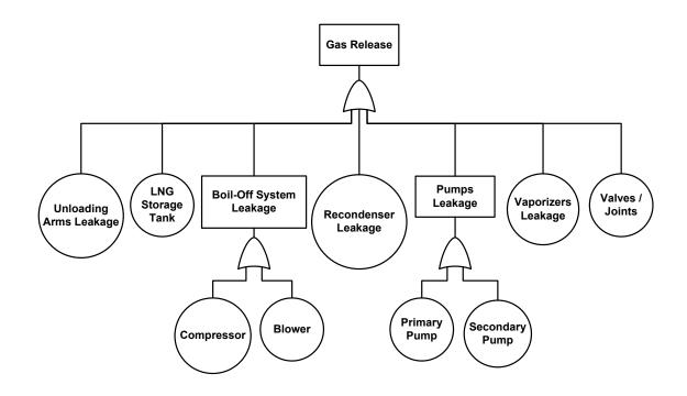
Figure 31. Fault tree for gas release during re-gasification process
