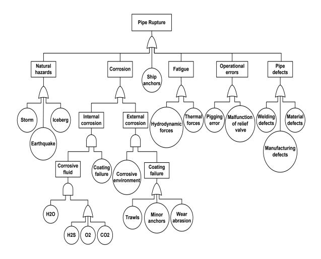
Figure 18. Fault tree of sub-sea pipe rupture
