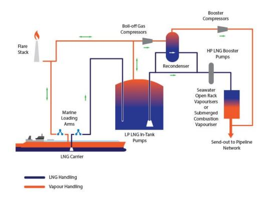
Figure 12. Schematic of LNG re-gasification facilities (www.ema.gov.sg)
