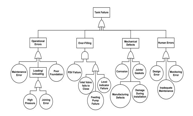
Figure 38. Fault tree of undesired release from storage tanks
