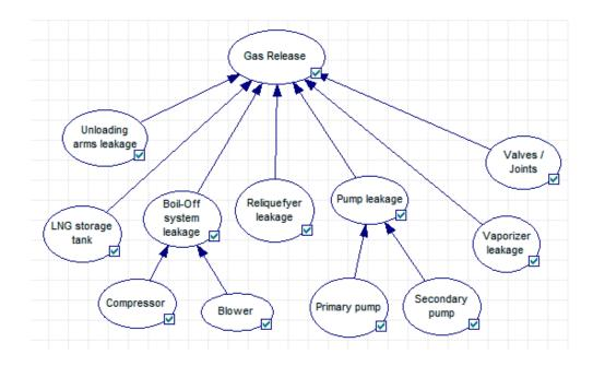
Figure 32. Bayesian network for gas release during re-gasification process
