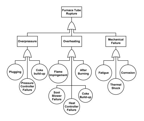
Figure 41. Fault tree of undesired release from a fired furnace
