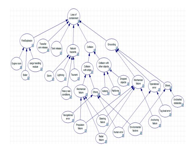
Figure 36. Bayesian network for crude oil release during shipping
