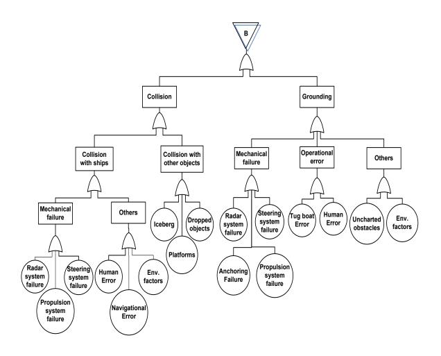
Figure 35. Fault tree for crude oil release during shipping (Part B)
