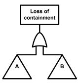
Figure 27. Fault tree for LNG release during shipping
