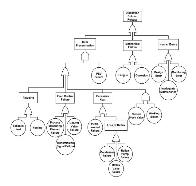
Figure 40. Fault tree of undesired release from an atmospheric distillation column
