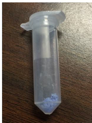
Figure 1. Dried CuHARS product. CuHARS was synthesized and dried as indicated in Section 2. A yield of 5 mg of blue product is shown in the bottom of a 2 mL plastic tube.
