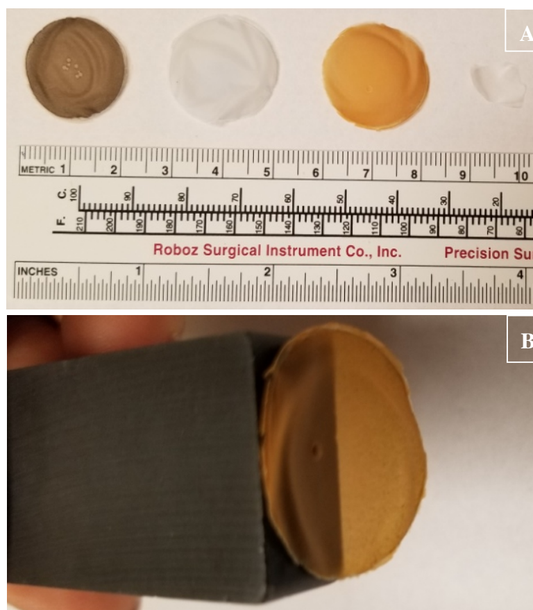
Figure 4. Cellulose matrices for materials integration. Panel (A) cellulose matrix at the macroscale, showing from left to right, cellulose biohybrids incorporating CuONPs, CuHARS, \text{Fe}_2\text{O}_3\text{NPs}/\text{CuHARS} , and cellulose alone, respectively. Metric scale below the matrix discs indicates a diameter of approximately 2 cm for each disc. The 4th sample (rightmost sample) is a fragment of the constructed cellulose matrix alone. Panel (B) magnetic susceptibility of materials incorporating \text{Fe}_2\text{O}_3\text{NPs}/\text{CuHARS} . Cellulose matrix sample incorporating susceptible \text{Fe}_2\text{O}_3\text{NPs} is suspended by a permanent bar magnet; the diameter of disc is same as shown in panel (A) (=2 cm).
